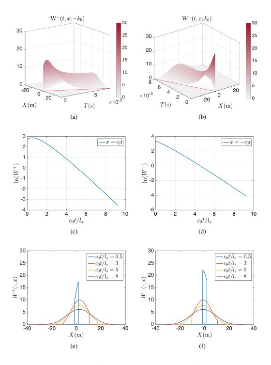
Fig. 4.3 Analytical solutions of W<sup>±</sup> in the time-space domain: (a) W<sup>+</sup>(t,x) (red line:  $x = c_0 t$ ), (b) W<sup>-</sup>(t,x) (red line:  $x = -c_0 t$ ), (c) ln(W<sup>+</sup>) on  $x = c_0 t + \Delta x$ , (d) ln(W<sup>-</sup>) on  $x = -c_0 t + \Delta x$ , (e) W<sup>+</sup>(·,x) for four time instants, (f) W<sup>-</sup>(·,x) for four time instants t = 0.4 ms, 2.6 ms, 4.4 ms and 7 ms, which correspond respectively to  $c_0 t / l_s(k_0) = 0.3$ , 3, 5 and 8.
