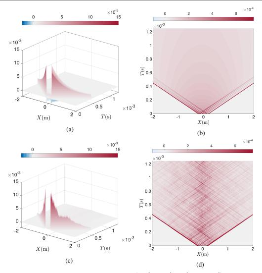
Fig. 4.9 Energy density in the time-space domain  $(t \in [0, 2 \text{ ms}], x \in [-2 \text{ m}, 2 \text{ m}])$  obtained by (a) (b): analytical Wigner measure  $E[W_a]$ , (c) (d): average of 10 numerical wave fields  $\mathbb{E}[E[u_{h\Delta t}]]$
