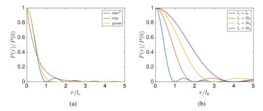
Fig. 4.1 (a) normalized sinc<sup>2</sup>, exponential and gaussian covariance functions, (b) sinc<sup>2</sup> function with different correlation lengths
