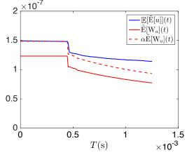
Fig. 4.10 Comparison of the evolution of energy in time obtained by analytical/numerical solutions:  $\mathbb{E}[\tilde{\mathbb{E}}[u_{h\Delta t}]]$  (blue solid line),  $\tilde{\mathbb{E}}[W_a]$  (red solid line),  $\alpha \tilde{\mathbb{E}}[W_a]$  (red dashed line)
