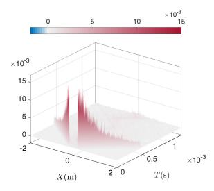
Fig. 4.8 Energy density in the time-space domain ( $t \in [0, 2 \text{ ms}], x \in [-2 \text{ m}, 2 \text{ m}]$ ) obtained by one realization of numerical wave fields  $E[u_{h\Delta t}]$
