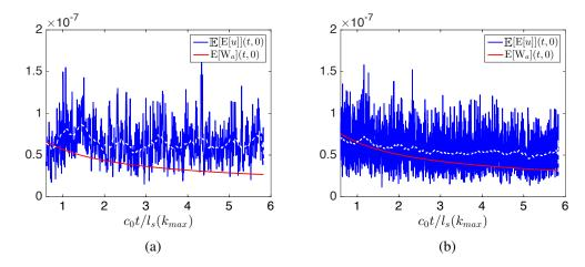
Fig. 4.15 Comparison of total energy obtained by analytical/averaged numerical solutions in time for x = 0 (white dashed line: smoothed value of  $\mathbb{E}[E(u_{h\Delta t})](t,0)$ ): (a)  $\varepsilon = 0.04$ , (b)  $\varepsilon = 0.008$
