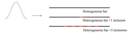
Fig. 2.4 Model for homogeneous or heterogenous bars (black zone:  $E_1$ , red zone:  $E_2$ )
