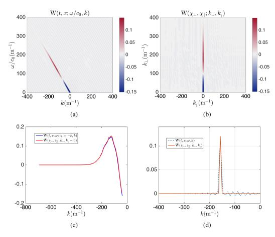
Fig. F.2 Wigner transform for coherent forward wave: (a)  $W_{\varepsilon}[u_{\varepsilon}](t,x;\omega,k)$  for  $(t=t_0,x=x_0)$ , (b)  $\tilde{W}_{\varepsilon}[\tilde{u}_{\varepsilon}](\chi_{\perp},\chi_{\parallel};k_{\perp},k_{\parallel})$  for  $(\chi_{\perp}=\frac{1}{\sqrt{2}}(c_0t_0-x_0),\chi_{\parallel}=\frac{1}{\sqrt{2}}(c_0t+x_0))$ , (c) values along the characteristic line, (d) values in the line perpendicular to the characteristic line for  $k=k_{max}$
