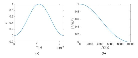
Fig. 2.3 Truncated ricker signal and its frequency spectrum (amplitude normalized to 1): (a) F(t), (b) |FFT(F)| (fast Fourier transform)
