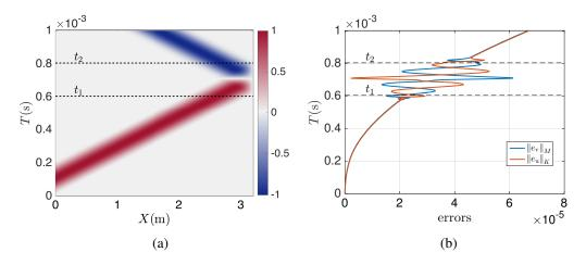
Fig. 2.7 Homogeneous media ( $\lambda/h = 32$ ): (a) velocity fields v(t,x), (b)  $||e_v||_M(t)$  and  $||e_u||_{K(\Omega)}(t)$
