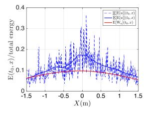
Fig. 4.11 Comparison of energy in time obtained by analytical/numerical solutions at  $t_1 = 0.5$  ms:  $\mathbb{E}[E[u_{h\Delta t}]]$  averaged in ten realizations (blue dashed line),  $\mathbb{E}[E[u_{h\Delta t}]]$  averaged in a local time-space domain and in ten realizations (blue solid line),  $E[W_a]$  (red line)
