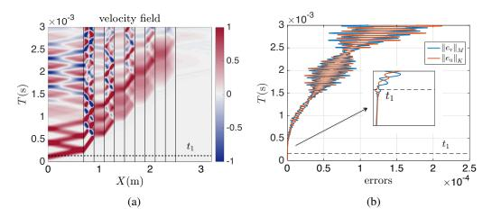
Fig. 2.9 Heterogeneous media with five inclusions ( $\lambda_2/h = 32$ ): (a) velocity fields v(t,x), (b)  $||e_v||_M(t)$  and  $||e_u||_{K(\Omega)}(t)$
