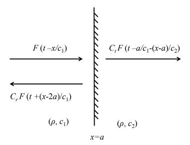
Fig. 2.5 Incident, reflected and transmitted waves
