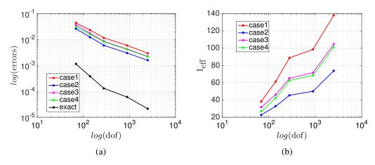
Fig. 2.11 Error estimation in the homogeneous case: (a) exact errors and estimated errors (log-log graph), (b) effectivity index (semi-log graph)
