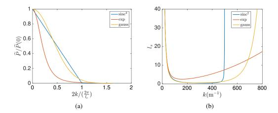
Fig. 4.4 Normalized power spectral density and mean free path for different correlation models: (a)  $\widehat{P}(2k)$ , (b)  $l_s(k)$  (parameters:  $\varepsilon = 0.04, l_c = 6$  mm)
