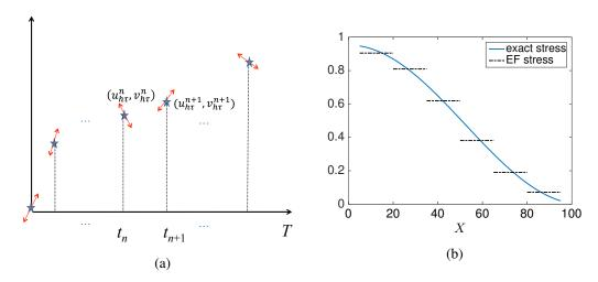
Fig. 2.1 (a) finite element solutions  $(\mathbf{u}_{h\Delta t}^n, \mathbf{v}_{h\Delta t}^n)$  in time, (b) exact and finite element stress in space
