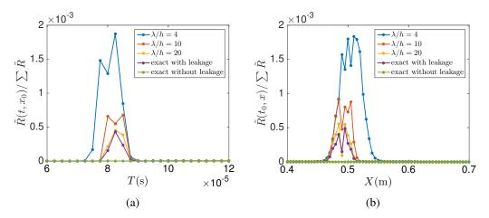
Fig. 3.16 Comparison of residual errors between numerical solutions and exact solutions: (a)  $\tilde{R}(t,x_0)$  for  $x_0 = 0.4$  m, (b)  $\tilde{R}(t_0,x)$  for  $t_0 = 0.1$  ms
