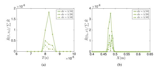
Fig. 3.17 Comparison of residual errors between three exact solutions with different discretizations: (a)  $\tilde{R}(t,x_0)$  for  $x_0=0.4$  m, (b)  $\tilde{R}(t_0,x)$  for  $t_0=0.1$  ms
