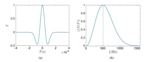
Fig. 3.4 Ricker signal and its frequency spectrum: (a) F(t), (b) |FFT(F)|
