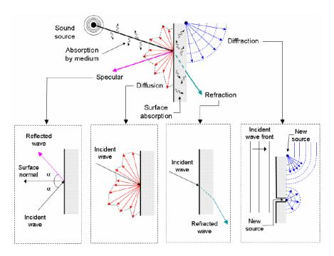
Fig. 1.4 Acoustic wave propagation phenomena: specular reflection, diffuse reflection, refraction and diffraction [84]
