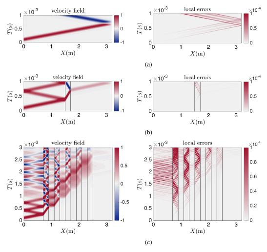
Fig. 2.6 Numerical results of velocity fields v(t,x) and local errors  $\frac{1}{2}\left\{\rho e_v^2 + E(\partial_x e_u)^2\right\}(t,x)$  (normalized by total energy  $\int_0^L \frac{1}{2}\left\{\rho v^2 + E(\partial_x u)^2\right\}dx = \text{constant}, \forall t$ ) for: (a) the homogeneous bar  $(\lambda/h=32)$ , (b) the heterogeneous bar with one inclusion  $(\lambda_1/h=278,\lambda_2/h=32)$ , (c) the heterogeneous bar with five inclusions  $(\lambda_1/h=278,\lambda_2/h=32)$
