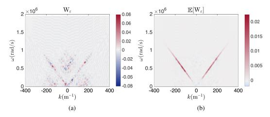
Fig. 4.18 Computation of Wigner transform for incoherent waves in random media: (a)  $W_{\varepsilon}[u_{h\Delta t}](t_0, x_0; \omega, k)$ , (b)  $\mathbb{E}[W_{\varepsilon}[u_{h\Delta t}]]$  (averaged in time-space and in 10 realizations)
