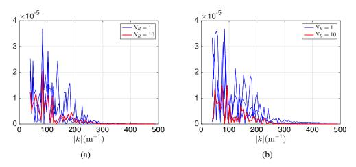
Fig. F.4 Residual errors in  $\omega = \pm c_0 k$  for incoherent wave: (a)  $|\tilde{\mathbf{R}}_T^{\rm sd}|$ , (b)  $|\tilde{\mathbf{R}}_{TS}^{\rm sd}|$
