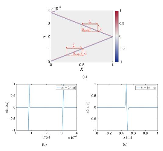
Fig. 3.9 Wave displacement: (a) u(t,x) in the whole computed time-space domain (with two computation regions for Wigner transform at two points A  $(t_A, x_A)$  and B  $(t_B, x_B)$ ), (b)  $u(t, x_0)$  for  $x_0 = 0.4$  m, (c)  $u(t_0, x)$  for  $t_0 = 0.1$  ms
