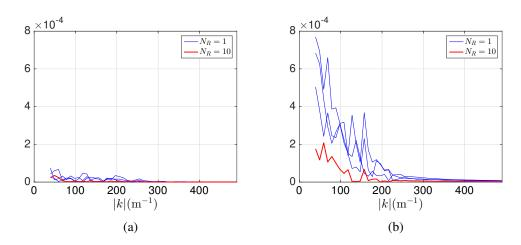
Fig. 4.21 Residual errors along  $\omega = \pm c_0 k$  for coherent wave: (a)  $|\mathbf{R}^+|$ , (b)  $|\mathbf{R}^-|$
