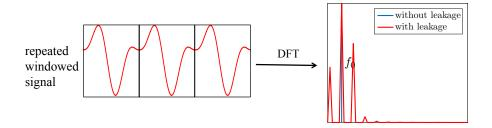
Fig. B.4 Example of the DFT of the periodic signal presented in fig. B.1: sampled signal with a hann window function and its DFT
