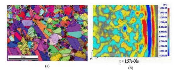
Fig. 1.1 (a) polycrystalline microstructure, (b) simulation of quasi-P wave propagation in polycristals (by MSSMat, CentraleSupélec)
