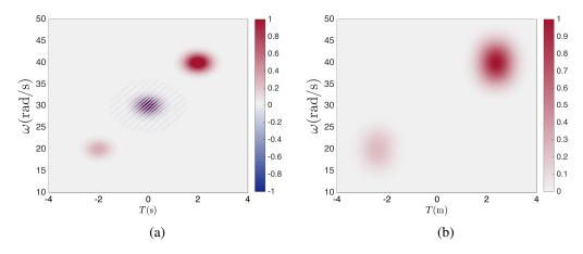
Fig. E.1 Comparison of Wigner transform and spectrogram of sum of two gaussian signal: (a) Wigner transform, (b) spectrogram  $[F](t;\omega)$
