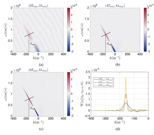
Fig. 3.8 W[u]( $t,x;\omega,k$ ) for ( $t_0,x_0$ ) at wave front with: (a) ( $\zeta_t,\zeta_x$ ) = ( $2T_{max},2\lambda_{max}$ ), (b) ( $\zeta_t,\zeta_x$ ) = ( $4T_{max},4\lambda_{max}$ ), (c) ( $8T_{max},8\lambda_{max}$ ); (d) their value at the line perpendicular to  $\omega=-c_0k$  for the maximum frequency  $k=-k_{max}$
