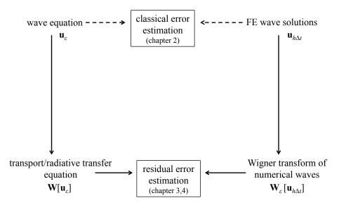
Fig. 1.6 Principle of the two a posteriori error estimations considered in this thesis
