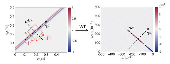
Fig. F.1 The rotational coordinates in the time-space domain (with u(t,x) of a forward wave) and in phase space (with  $W(t_0,x_0;\omega,k)$ ):  $(\chi_{\perp},\chi_{\parallel})=(\frac{1}{\sqrt{2}}(c_0t-x),\frac{1}{\sqrt{2}}(c_0t+x)), \ (k_{\perp},k_{\parallel})=(\frac{1}{\sqrt{2}}(\frac{\omega}{c_0}-k),\frac{1}{\sqrt{2}}(\frac{\omega}{c_0}+k))$
