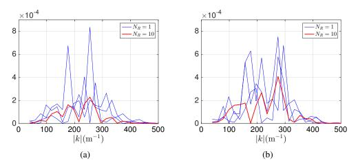
Fig. F.5 Filtered residual errors in  $\omega = \pm c_0 k$  for coherent forward waves: (a)  $\left| \tilde{\mathbf{R}}_1^{\mathrm{sd}} * * \tilde{\mathbf{W}} [\tilde{h}_{\chi_{\perp}} \tilde{h}_{\chi_{\parallel}}] \right|$ , (b)  $\left| \tilde{\mathbf{R}}_2^{\mathrm{sd}} * * \tilde{\mathbf{W}} [\tilde{h}_{\chi_{\perp}} \tilde{h}_{\chi_{\parallel}}] \right|$
