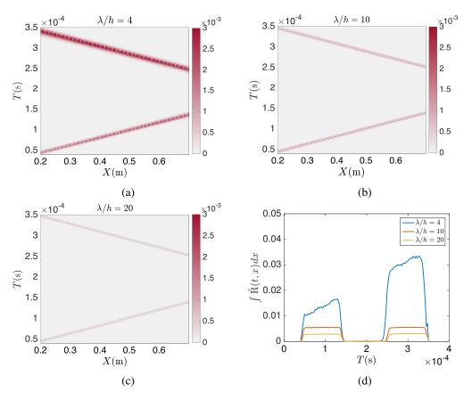
Fig. 3.15  $\tilde{R}(t,x)/\sum \tilde{R}$  for numerical solutions with different mesh size and time step: (a)  $\lambda/h=4$ , (b)  $\lambda/h=10$ , (c)  $\lambda/h=20$ , (d)  $\int_{x\in[0.2,0.7]}\tilde{R}(t,x)dx$
