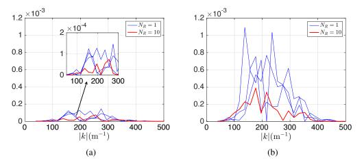
Fig. F.6 Filtered residual errors in  $\omega = \pm c_0 k$  for incoherent waves: (a)  $\tilde{\mathbf{R}}_1^{\mathrm{sd}} * * \tilde{\mathbf{W}} [\tilde{h}_{\chi_{\perp}} \tilde{h}_{\chi_{\parallel}}]$ , (b)  $\tilde{\mathbf{R}}_2^{\mathrm{sd}} * * \tilde{\mathbf{W}} [\tilde{h}_{\chi_{\perp}} \tilde{h}_{\chi_{\parallel}}]$
