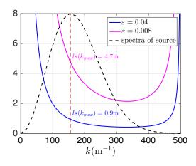
Fig. 4.6 Mean free path  $l_s(k)$  (parameters:  $\varepsilon = 0.04, 0.008, l_c = 6$  mm)
