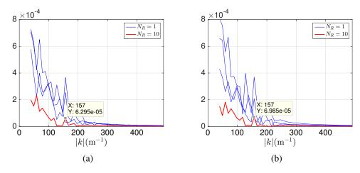
Fig. 4.20 Residual errors along  $\omega = \pm c_0 k$  for coherent wave: (a)  $|\mathbf{R}_T^{\rm sd}|$ , (b)  $|\mathbf{R}_{TS}^{\rm sd}|$
