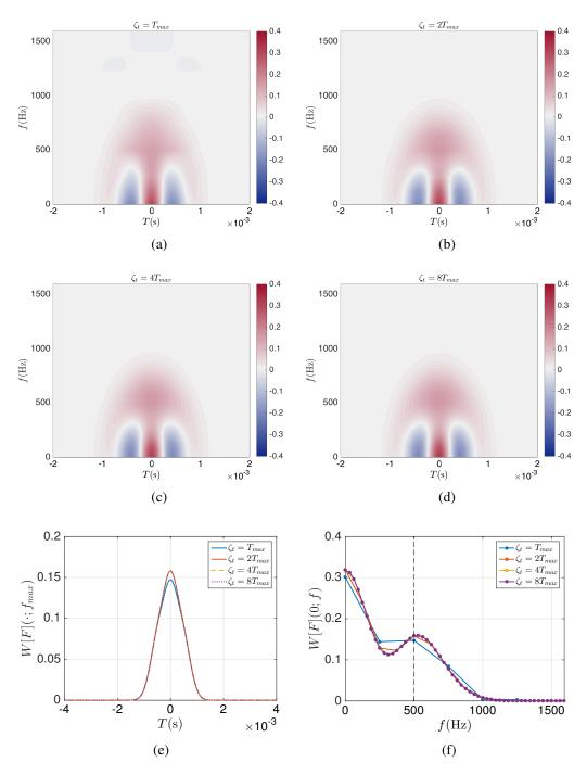
Fig. 3.5 Wigner transform of ricker signal W[F](t; f) for (a)  $\zeta_t = T_{max}$ , (b)  $\zeta_t = 2T_{max}$ , (c)  $\zeta_t = 4T_{max}$ , (d)  $\zeta_t = 8T_{max}$ ; comparison of (e) W[F](t;  $f = f_{max}$ ) and (f) W[F](t = 0; f) for the four considered values of  $\zeta_t$
