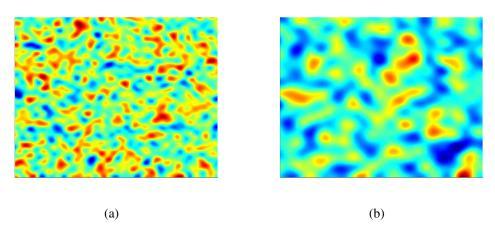
Fig. 4.2 One realization of 2D random media generated by the covariance function  $sinc^2$  with different correlation lengths: (a)  $l_c = l_0$ , (b)  $l_c = 2l_0$
