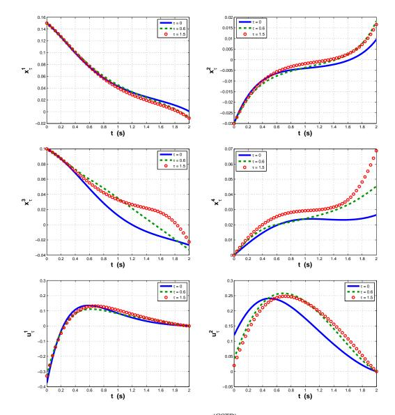
Figure 6.1: Optimal quantities of  $(\mathbf{OCP})^{(\text{CSTR})}_{\tau}$  for different delays  $\tau$ .
