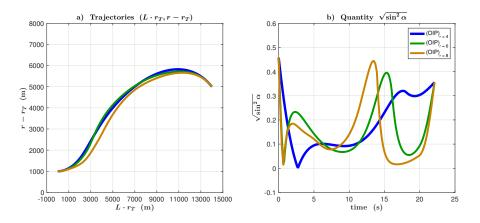
Figure 6.8: Two-dimensional trajectories and stability constraints of  $(OIP)_{\tau}^{a}$ .
