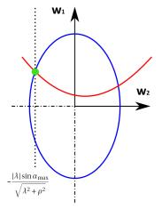
$$\begin{cases} w_1 = \cos \alpha_{\max} & \text{Figure 3.4} \\ w_2 = \frac{|\lambda| \sin \alpha_{\max}}{\sqrt{\lambda^2 + \rho^2}} & \text{, if } \frac{\lambda}{D_a} < 0 \\ & (3.33) & \text{parabola a} \end{cases}$$
