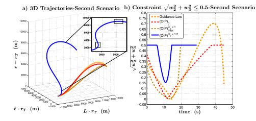
Figure 4.8: Trajectories and constraints of the second scenario, with minimal time. The black boxes within the subplot of Figure a) show changes of local chart.
