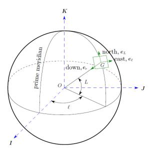
Figure 2.1: Graphical relations between frame (I, J, K) and frame  $(e_L, e_\ell, e_r)$ .
