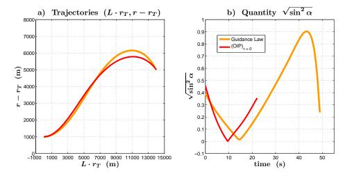
Figure 6.4: Two-dimensional trajectories and stability constraints for the derivative of the guidance law (4.22)-(4.23) and (**OIP**)<sup>*a*</sup><sub> $\tau=0$ </sub>.
