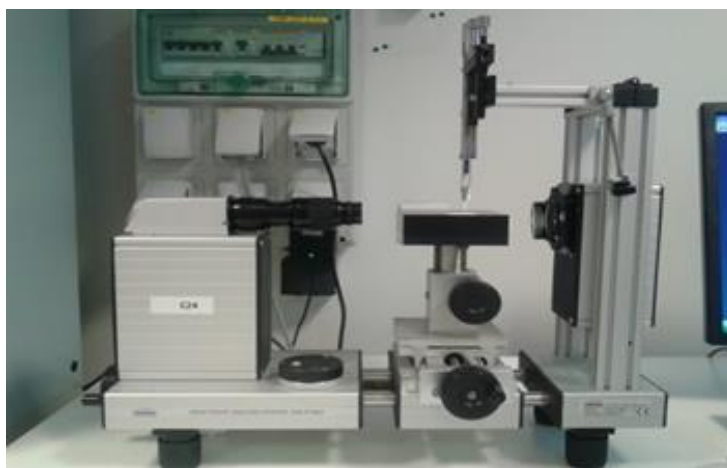
Figure 2-11. Krüss DSA10-Mk2 contact angle machine.
