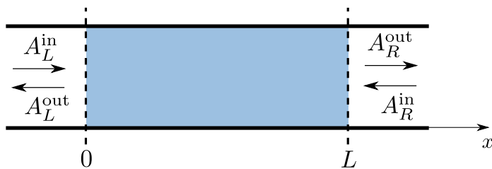
Figure 5.1: A scattering situation of a disordered wire of size L connected to two perfect leads. On each side, the wave function is the superposition of ingoing and outgoing plane waves.
