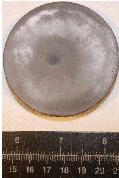
Figure III)31: Sample sized for ballistic test
