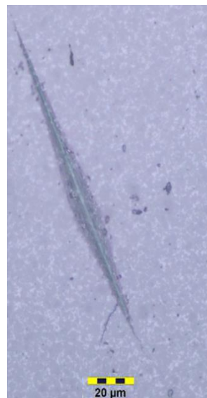
Figure II)10: Knoop imprint with 2kg load
