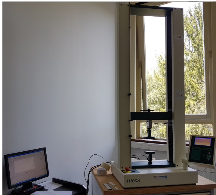
FIGURE 2.3 – Machine de traction uni-axiale Tinius Olsen.
