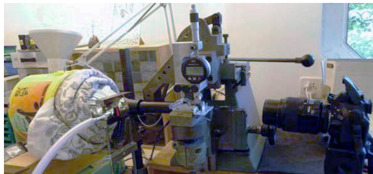
Figure 4.3 – Overview of the experimental device during aeraulic measurements. Compare with the scheme of the same device in Fig. 4.5. From left to right: the thermally insulated bottle (about 3L), the plug, the cock valve, the connection joint (with insulating foam), the vise immobilizing the instrumented mouthpiece, the digital dial gauge to which the artificial lip is attached, the micrometric adjustment screw, the frame of the old milling machine, the camera with macro lens (for the calibration of the optical sensors).
