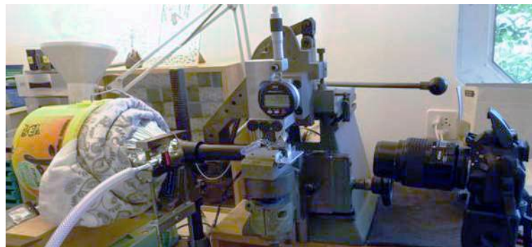
Figure 4.3 – Overview of the experimental device during aerodynamic measurements. Compare with the scheme of the same device in Fig. 4.5. From left to right: the thermally insulated bottle (about 3L), the plug, the cock valve, the connection joint (with insulating foam), the vise immobilizing the instrumented mouthpiece, the digital dial gauge to which the artificial lip is attached, the micrometric adjustment screw, the frame of the old milling machine, the camera with macro lens (for the calibration of the optical sensors).
