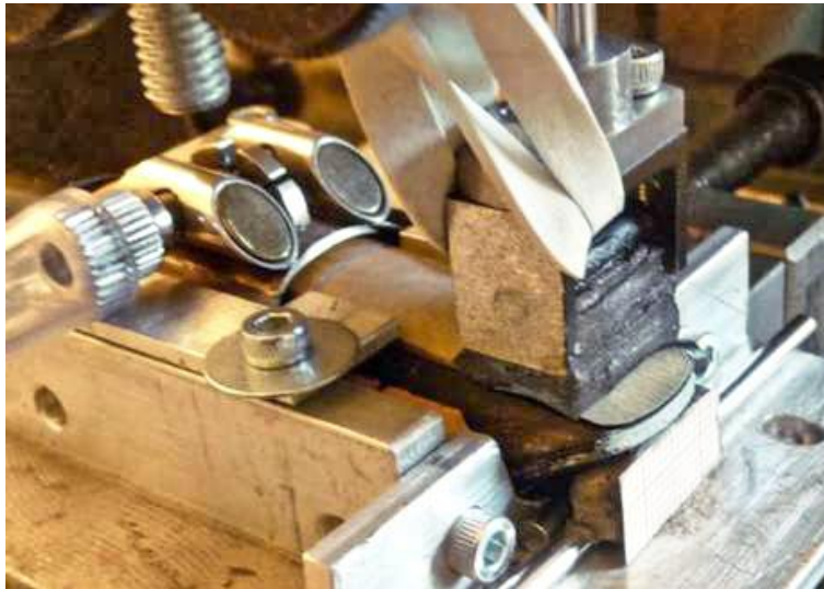
Figure 4.4 – View of the instrumented mouthpiece and the artificial lip in measurement situation. Observe the instrumented mouthpiece immobilized in the vise, one of the positioning stops (lateral and longitudinal) of the reed, the ligature, the reed, the millimeter scale, the artificial lip and its stirrup screwed to the spindle of a digital dial gauge. The elastic counterbalance the spring of the dial gauge, so as to press the spindle of the dial gauge against the micrometer screw.
