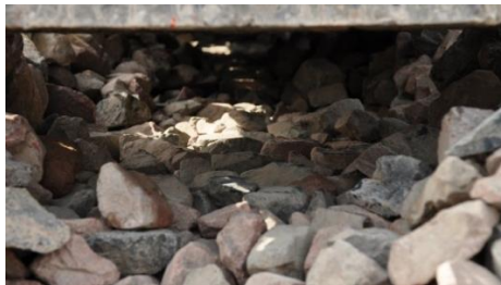
Figure 1.8 Compacted grains below the sleeper after a vibration test.
