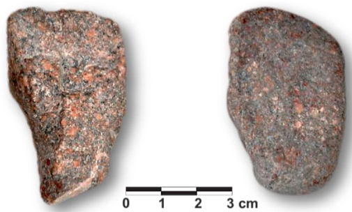
Figure 1.12 New grain (left) compared to a grain after a Micro-Deval test (right).
