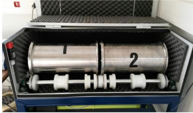
Figure 2.1 Micro-Deval device in the 3SR Laboratory, with larger cylinders adapted to ballast grains.
