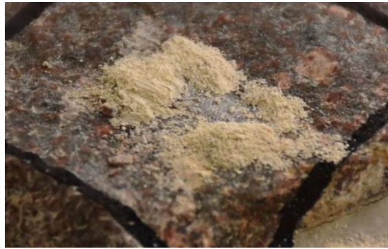
Figure 1.17 Wear produced by shearing two ballast grains in the BCR3D device along 200 cycles at 1.2 mm of amplitude. Fines can be expelled out of the interface or remain trapped within.
