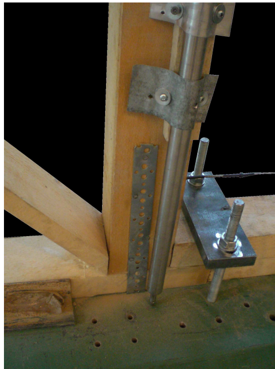
Fig. 5.12: Side supporting of the shear wall.
