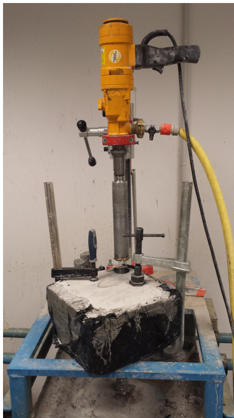
Figure 7.1: Sample manufacturing: example of the use of the coring machine.
