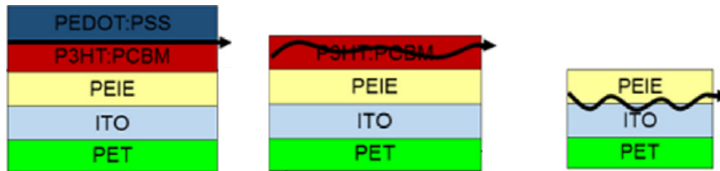
Figure 1.37: R2R inverted samples tested mechanically. Arrows represent the corresponding fracture path. Reproduced from [129].
