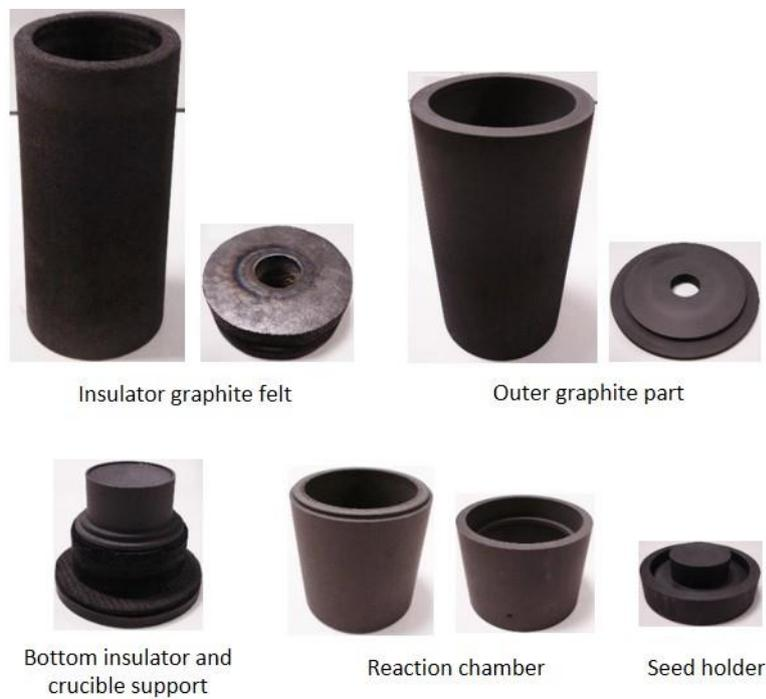
Figure 2.6: Main parts of the external graphite crucible used for experiments.
