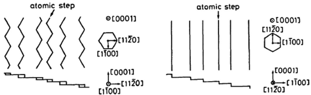
Figure 4.29: Configurations of steps on off-oriented (0001) faces toward  $[11-20]$  and  $[1-100]$ <sup>10</sup>. This description has been proposed on  $\alpha$ -SiC.
