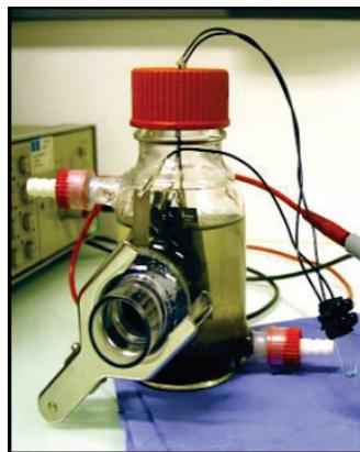
**Figure 2.1. MFC bottle with an air cathode.**
