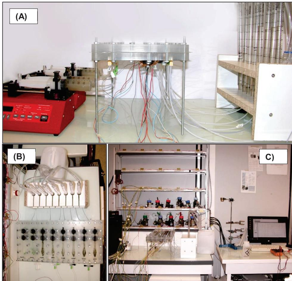
**Figure 2.4. Photography of the experimental set up.** (A) and (B) Images of the reactors. (c) Image of the reactor connected to a voltammeter and a computer to recorder the cell voltage as a function of the time.
