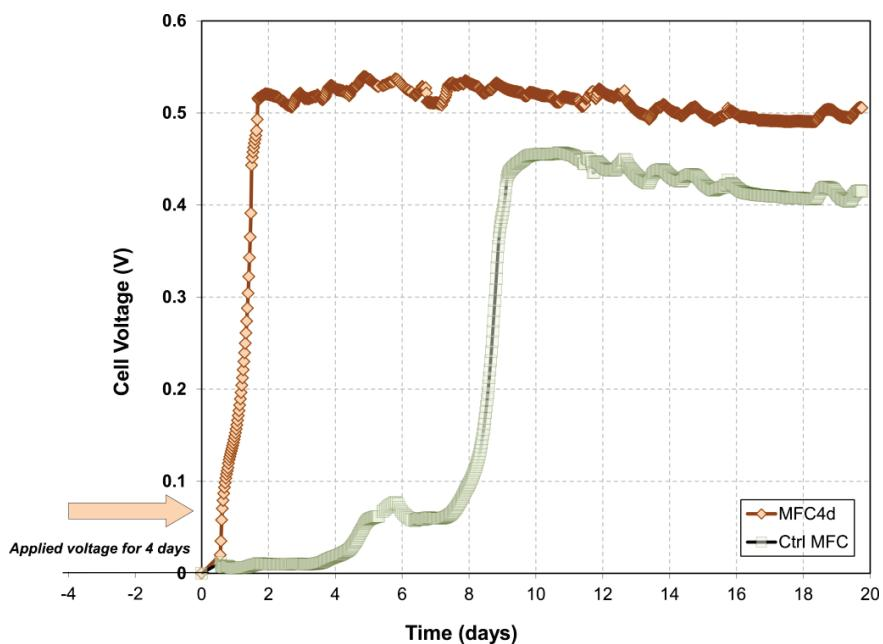
**Figure.1. Evolution of the microbial fuel cell voltage as a function of time after the applied voltage (MFC4d) and without preceding phase of applied voltage (CtrlMFC). The external resistance was set at 1000 Ohms.**
