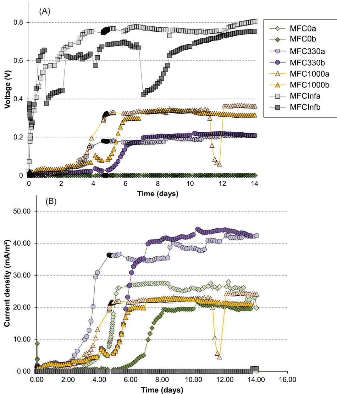
**Figure 3.4. Electricity production as a function of time of MFCs.** The experiment was performed in duplicate (a and b). The MFCs were set up with different external resistance: 1000 ohms (purple), 330 ohms (yellow), 0 ohms (green) and an infinite resistance (electrode are disconnected) (gray).
