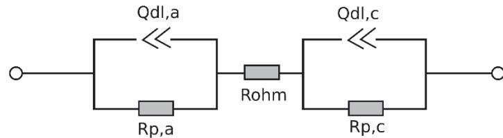
**Figure 6.2. Circuit model for impedance spectroscopy studies. Rohm corresponds to the ohmic resistances,  $R_{p,a}$  and  $R_{p,c}$  to the charge transfer resistances of respectively the anode and the cathode.**
