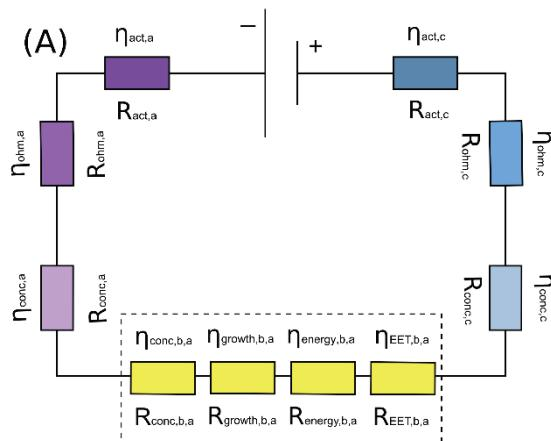
**Figure 1.3. Equivalent electrical circuit of a MFC.** Equivalent electrical circuit of a MFC with a bioanode and an abiotic cathode such as the MFC represented in the Figure 1.3. Each overpotential is associated to a resistance. Purple and blue resistances correspond respectively to the abiotic steps in the anodic and cathodic compartment. Yellow resistances corresponding to the biotic steps of the anodic biofilm.
