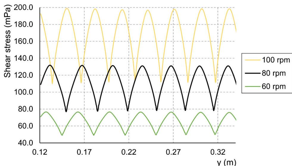
**Figure 6.6.** Shear stress in mPa in function of the y axis for a rotation velocity of 60, 80 or 100 rpm.
