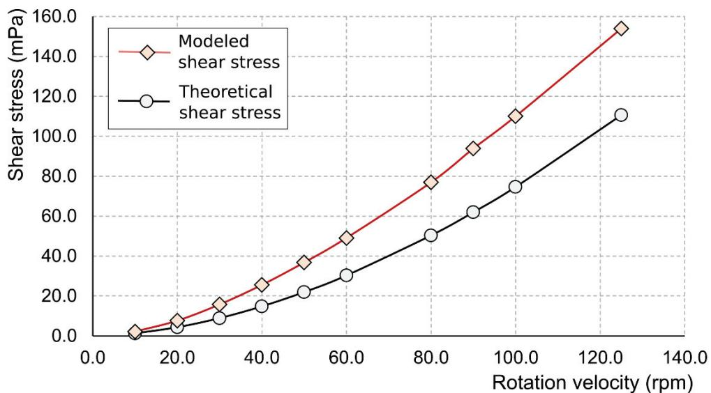
**Figure 6.7.** Shear stress in mPa on the anodic surface as a function of the rotation velocity. The dark curve represents the theoretical shear stress calculated by the equations (6.3), (6.4) and (6.5). The red curve is the shear stress measured using the model.
