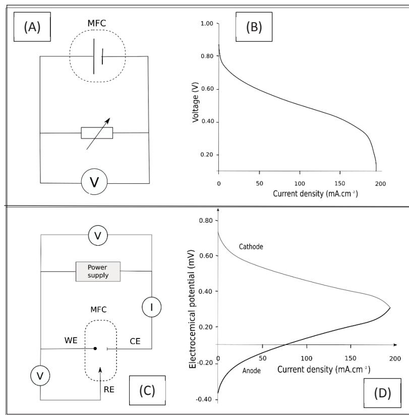
**Figure 2.6. Polarization curves.** (A) Method of measure with an adjustable resistance. (B) Voltage as a function of the current obtained by the method (B) or deduced from the curves (D). (C) Method of measure by linear voltammetry. (D) Potential of the anode and the cathode as a function of the current obtained by the method (C).
