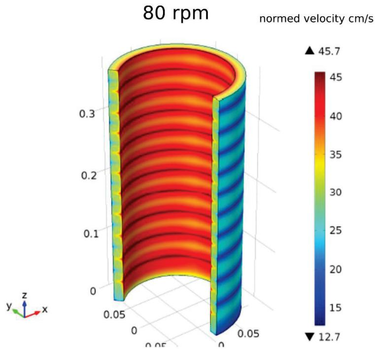
**Figure 6.5.** Flow regime at 80 rpm. The 3D graphic represents the normed velocity in  $\text{cm} \cdot \text{s}^{-1}$ . Taylor vortex can be observed at 80 rpm.
