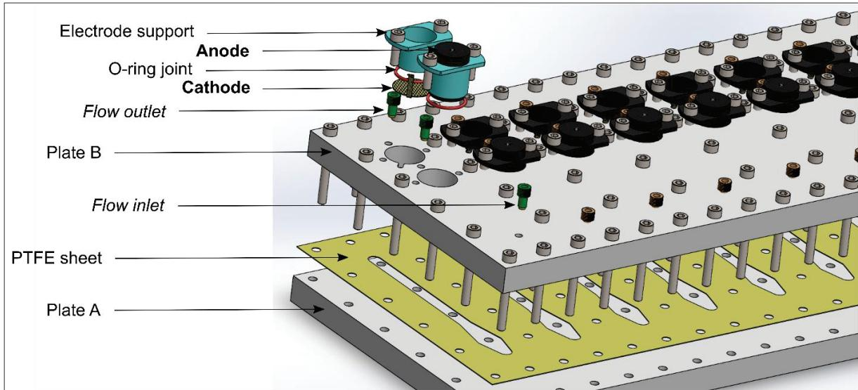
**Figure 2.3. Schematic of a multichannel MFC configuration**
