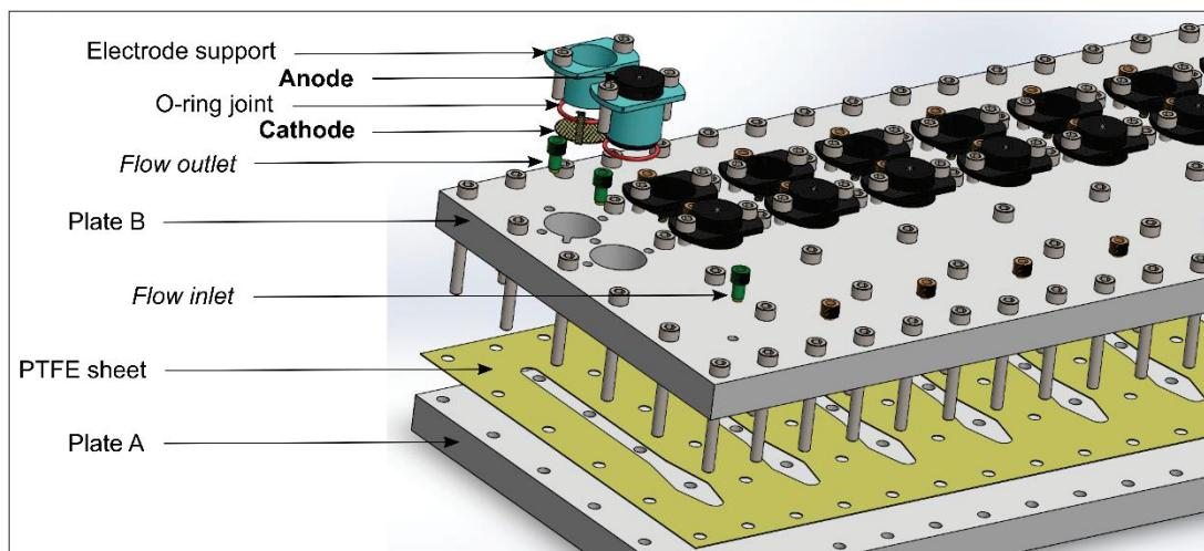
**Figure 4.1. Schematic of a multichannel MFC configuration**
