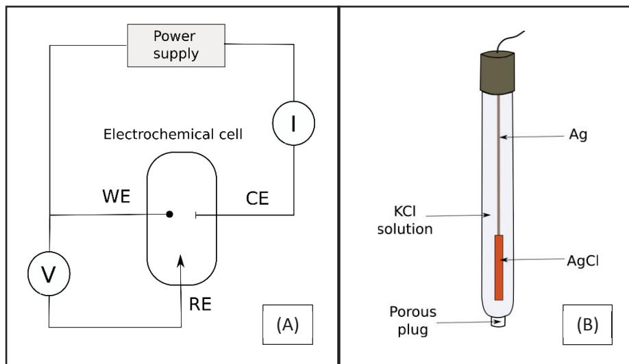
**Figure 2. 5. (A)** A schematic of a potentiostat representing the counter electrode (CE), the working electrode (WE), the reference electrode (RE), an ammeter (I) and a voltammeter (V). **(B)** A schematic of a silver chloride electrode.
