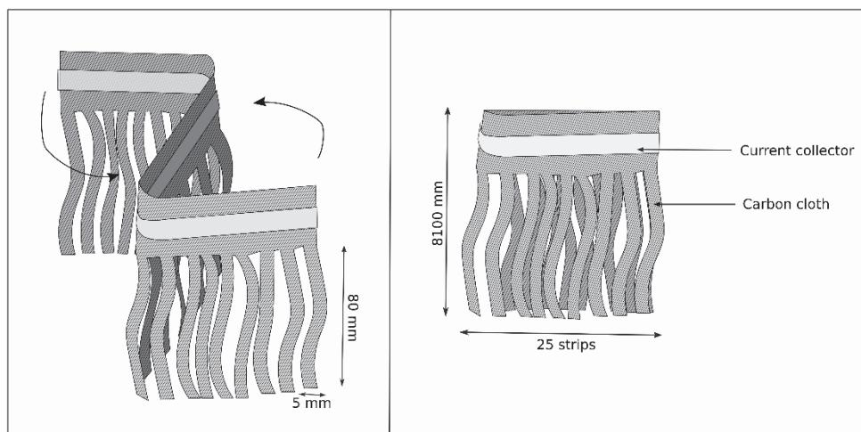
**Figure 3.1. Schematic of the anodes.** The anode was constituted of 25 carbon cloth strips of 80 x 5 mm. A titanium strip was used as the collector.
