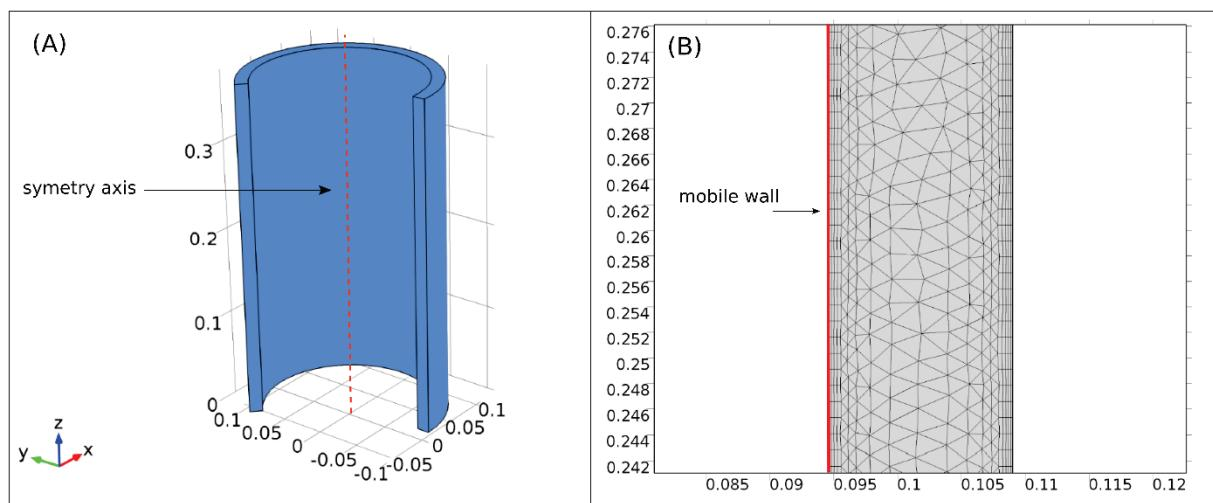
**Figure 6.3. Model geometry of the Taylor reactor. (A) 3D schematic of the reactor.** The symmetry axis is represented in red and is the origin of the x and y axis. The xyz dimensions are in meter. (B) The 2D model of the reactor. The space between the cylinders is represented by a rectangular area with a mobile wall. The mesh is represented. The axis are the dimensions x and y in meter.
