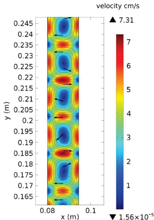
**Figure 6.9.** Flow normed velocity in x and y axis at 80 rpm
