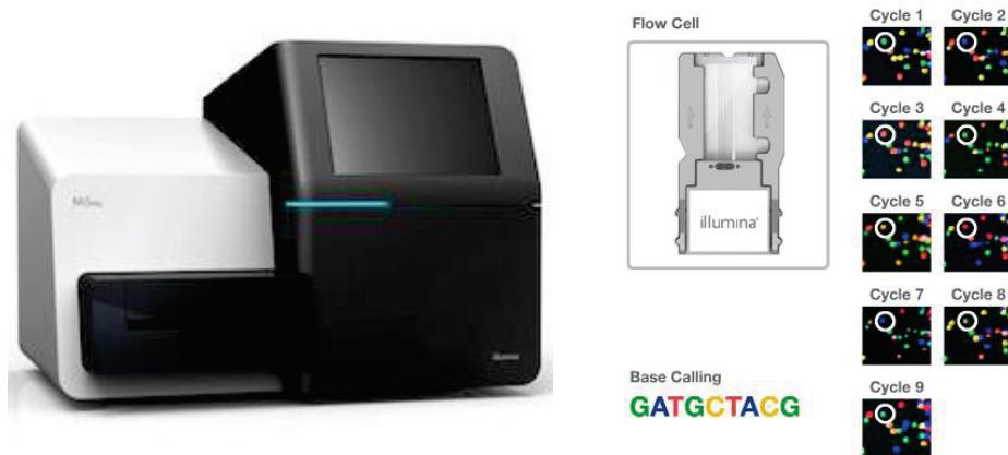
**Figure 2.9. MiSeq Illumina technology** (adapted from [www.illumina.com](http://www.illumina.com)). (A) Image of a MiSeq. (B) Image of a flow cell and the images taken at each cycle to detect the fluorescent signal to identify the bases.
