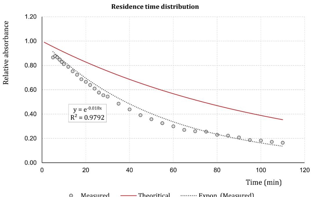
**Figure 6.8. Residence time distribution.** The red curve represents the theoretical distribution in a perfect mixed reactor. The points represent the experimental measured and the dotted curve represents the tendency curve from experimental points.
