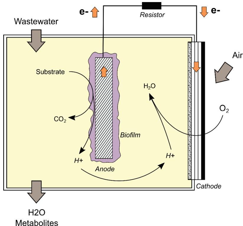
**Figure 1. Schematic of a Microbial Fuel Cell**
