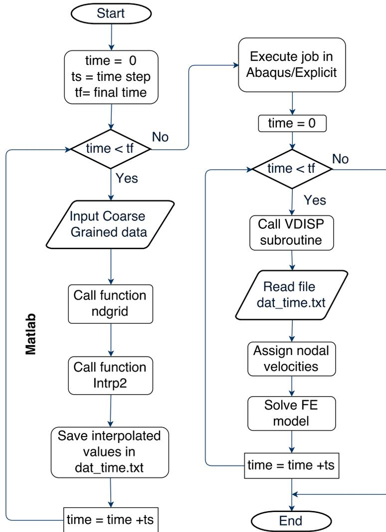
Figure 4.10: Flow chart block diagram describing the FEM simulation using CG results.
