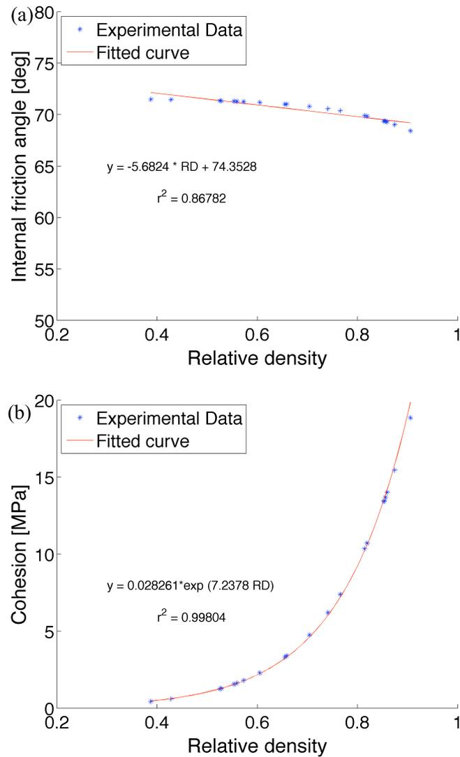
Figure 2.8: Shear failure parameters a) internal friction angle,  $\beta$  b) Cohesion,  $d$ .
