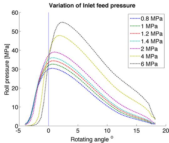
Figure 3.8: Effect of inlet feed pressure on the roll pressure
