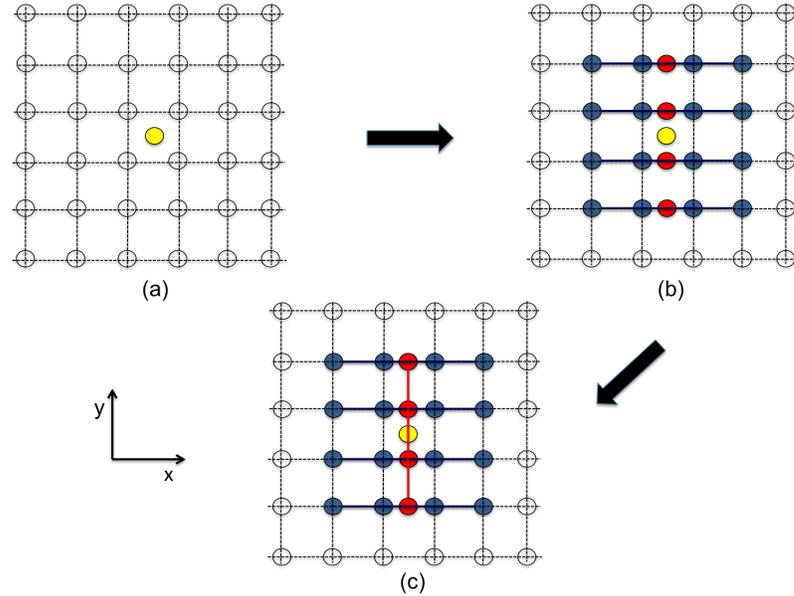
Figure 4.7: Schematic illustration of the Bicubic Convolution interpolation procedure. a) Initial point to be interpolated, b) First interpolation step along the x-direction. c) Final interpolation step along the y-direction
