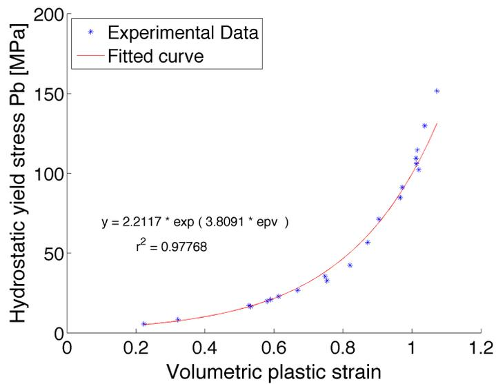
Figure 2.11: Hydrostatic compressive stress,  $P_b$  as a function of volumetric plastic strain
