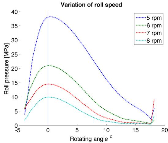
Figure 3.20: Effect of roll speed (using inlet feed velocity) on the roll pressure
