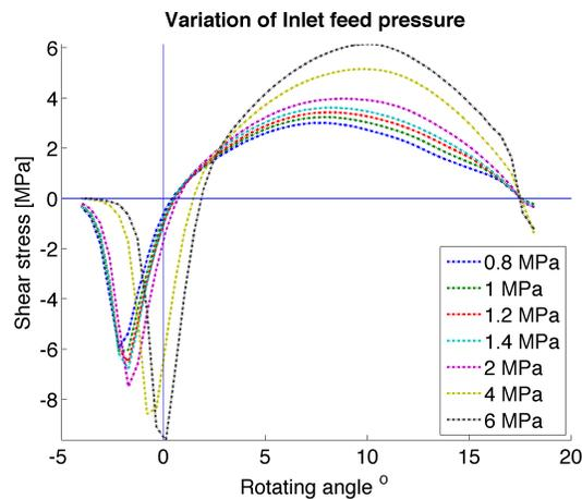
Figure 3.9: Effect of inlet feed pressure on the shear stress
