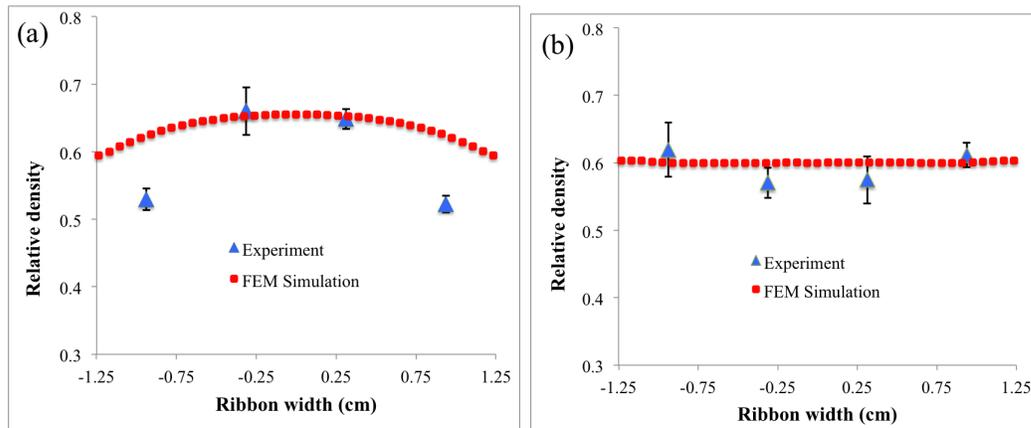
Figure 3.30: Ribbon's density distribution for a)cheek plates and b)rimmed-roll
