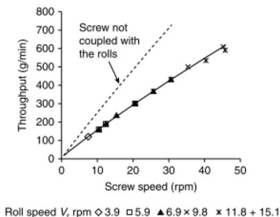
Figure 1.8: Screw throughput as a function of screw speed [47]
