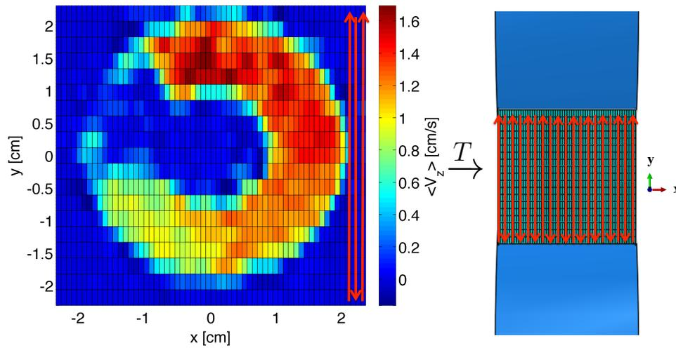
Figure 4.9: Schematic illustration of the procedure assigning axial inlet velocity interpolated values into the FE model. The red arrows shows the direction in which values are read in the data file and being assigned into the FE back nodes.
