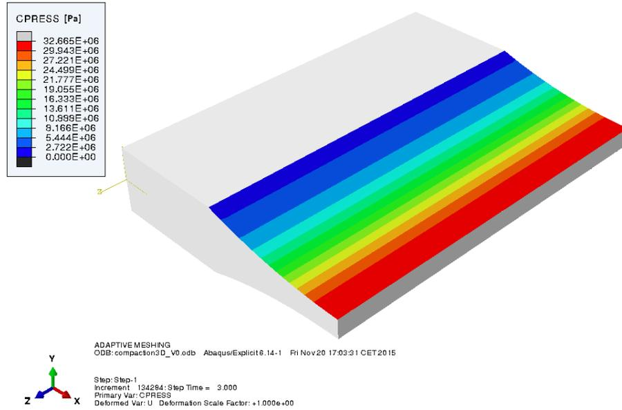
Figure 3.3: Reference FEM model results of roll contact pressure
