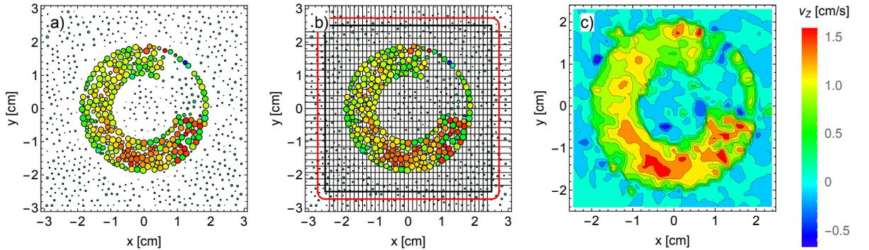
Figure 4.4: Schematic illustration of the coarse graining process (sub-figures left to right) along the x-y plane, with the particle direction of flow towards the reader and the screw rotating clockwise. The particles and field are coloured according to the axial component of the velocity  $v_z$ .
