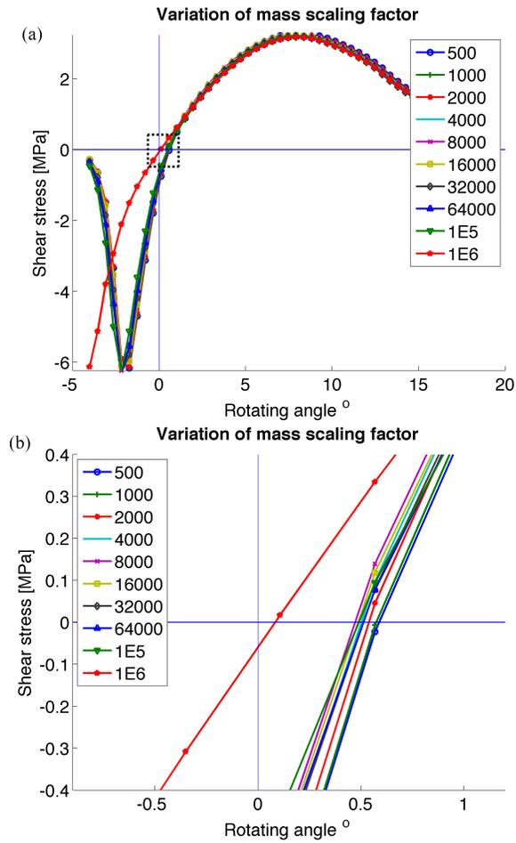
Figure 3.6: Effect of mass scaling on shear stress along rolling direction
