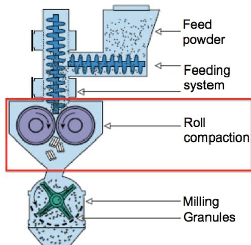
Figure 1.1: Scheme of a typical dry granulation process [20]
