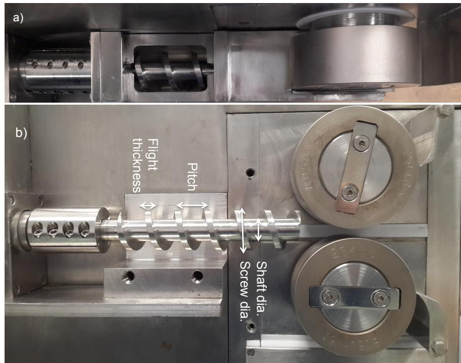
Figure 4.1: Komarek B050H roll compactor; a) Top view and b) Side view (w/o feed barrel and side seals)
