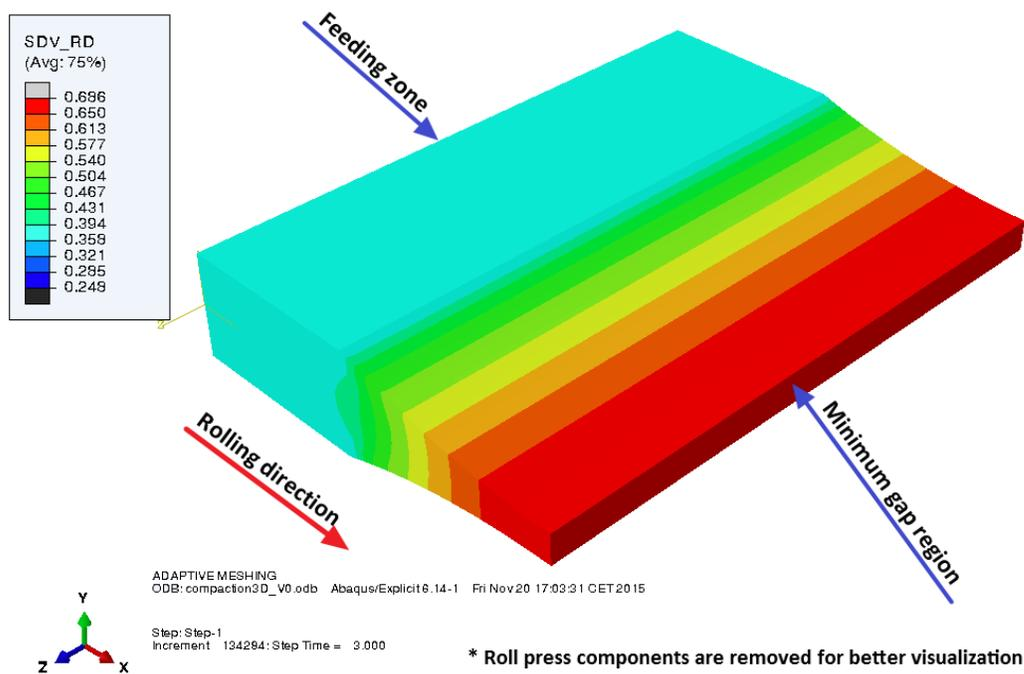
Figure 3.2: Reference FEM model results of relative density
