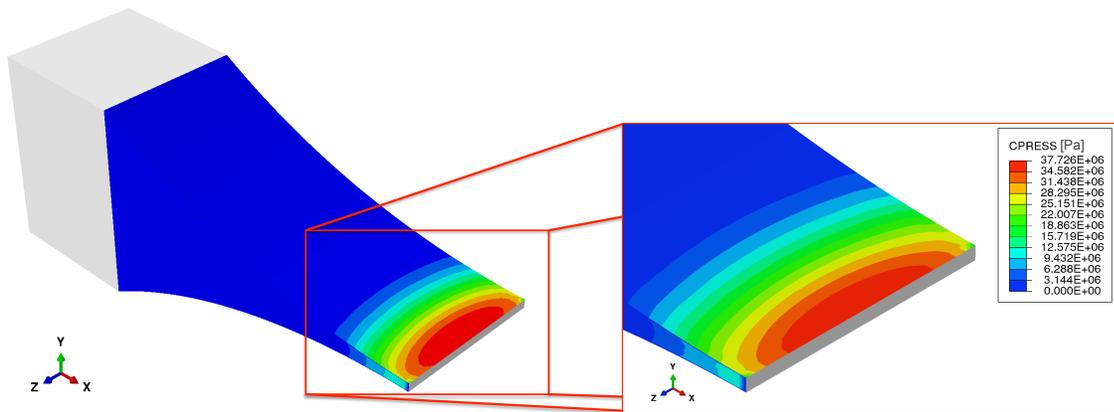
Figure 3.27: Contact pressure between powder and upper roll for cheek plates assembly
