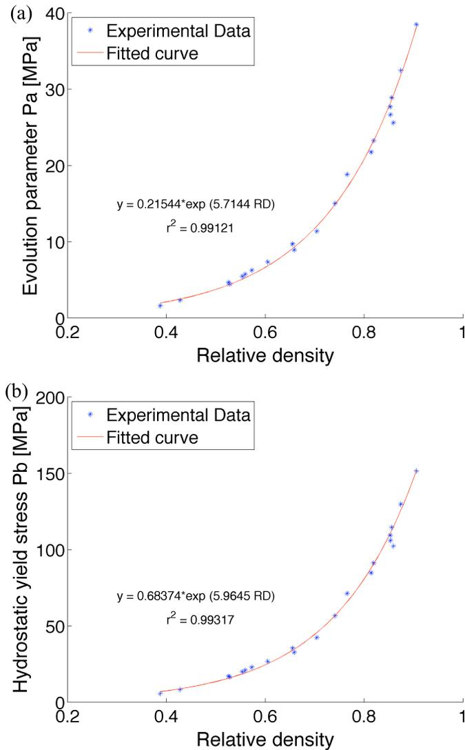
Figure 2.9: Cap parameters a)  $Pa$  and b)  $Pb$  as function of relative density.
