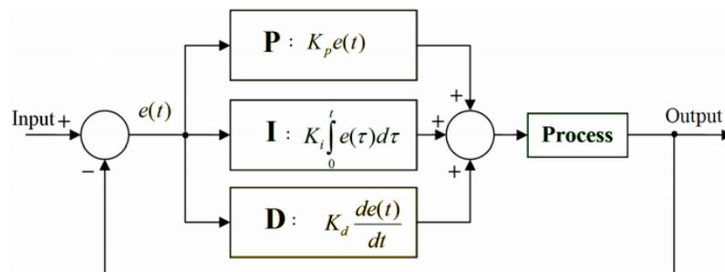
Figure 5.1: Closed-loop feedback single-output control using a PID controller [93].
