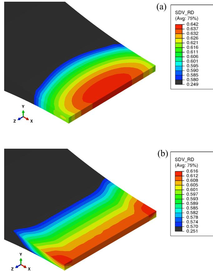
Figure 3.29: Relative density for the two sealing systems a)cheek plates and b)rimmed-roll
