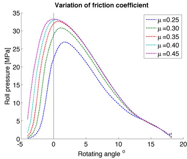
Figure 3.14: Effect of friction coefficient on the roll pressure
