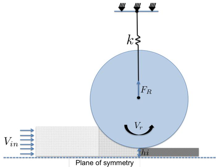
Figure 5.2: Scheme of floating roll
