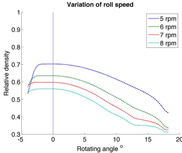
Figure 3.22: Effect of roll speed (using inlet feed velocity) on the roll powder’s relative density
