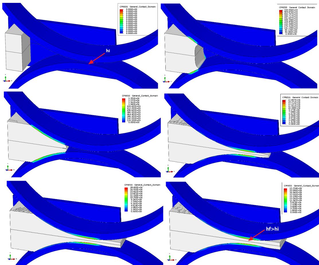
Figure 5.5: Powder flow and roll pressure during CEL modelling (Full model view by mirroring the symmetry planes).
