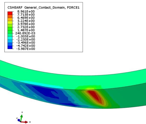
Figure 5.8: Resultant roll shear stress in CEL FEM model
