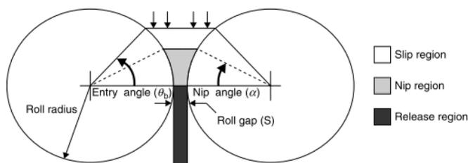
Figure 1.12: Schematic diagram of a typical roll compaction design [6]
