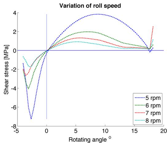
Figure 3.21: Effect of roll speed (using inlet feed velocity) on the shear stress
