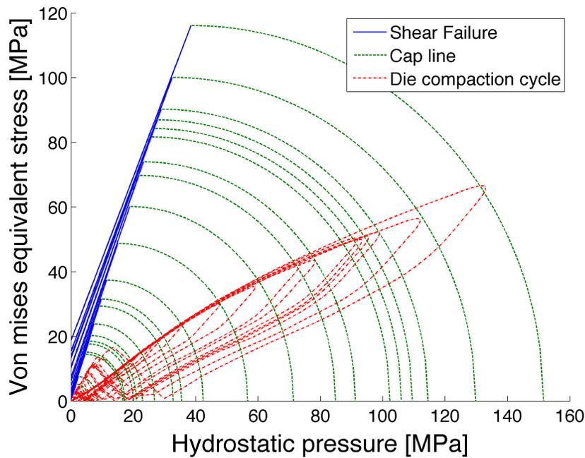
Figure 2.12: Experimental iso-density Drucker-Prager Cap
