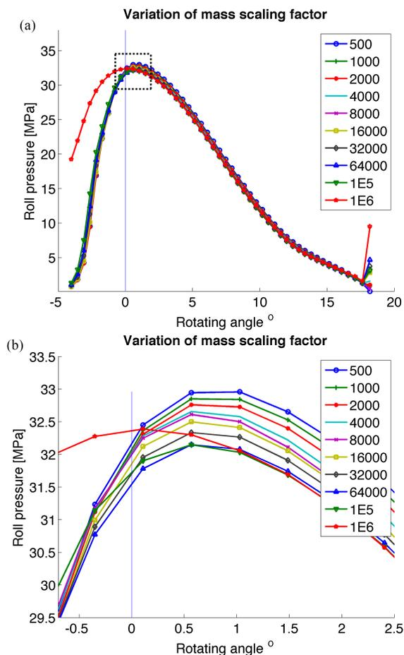
Figure 3.5: Effect of mass scaling on roll pressure along rolling direction
