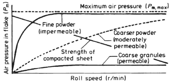
Figure 1.11: Effect of roller speed and permeability on air pressure in compacted sheet [53]
