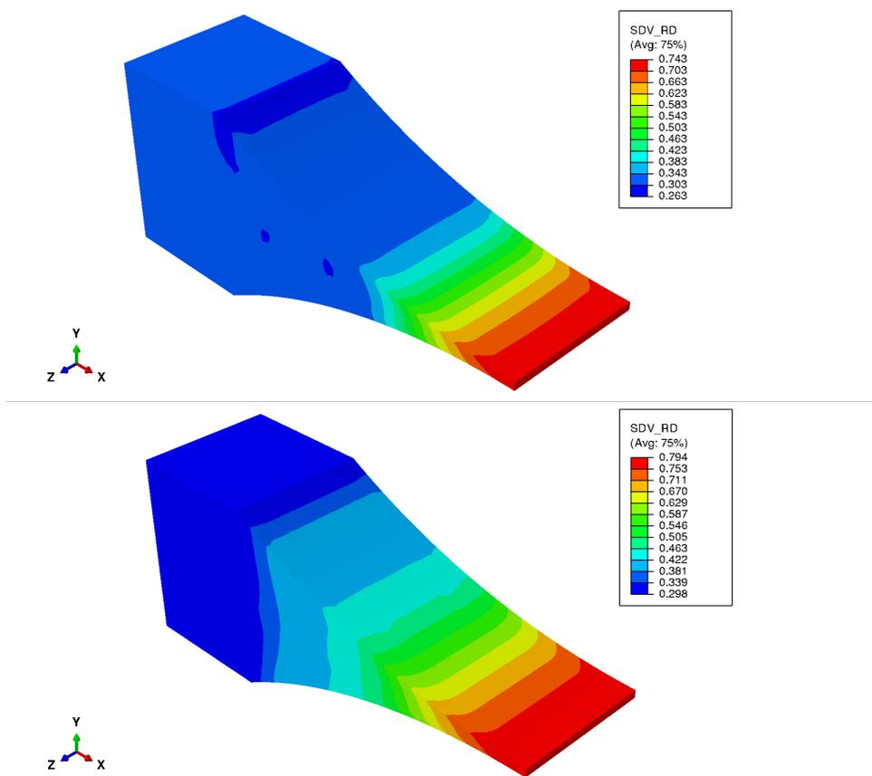
Figure 3.26: Resultant vertical stress,  $\sigma_{22}$  with a rimmed-roll for a) 6 kN/cm and b) 8 kN/cm roll separation force
