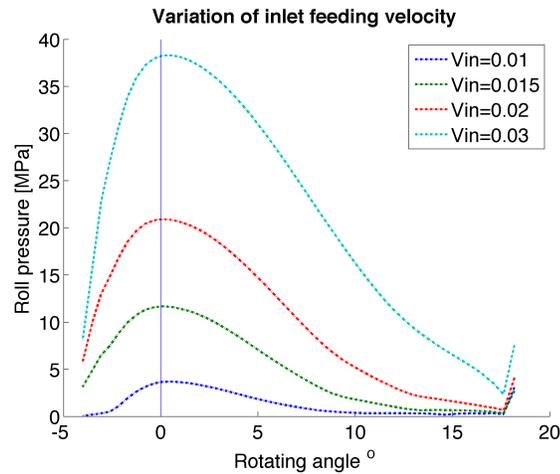
Figure 3.11: Effect of inlet feed velocity on the roll pressure
