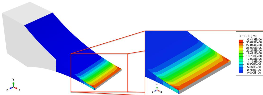
Figure 3.28: Contact pressure between powder and upper roll for rimmed-roll assembly
