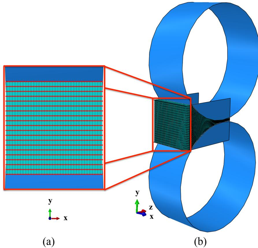
Figure 4.3: Visualization of the (a) Back inlet nodes and (b) Entire FEM model.
