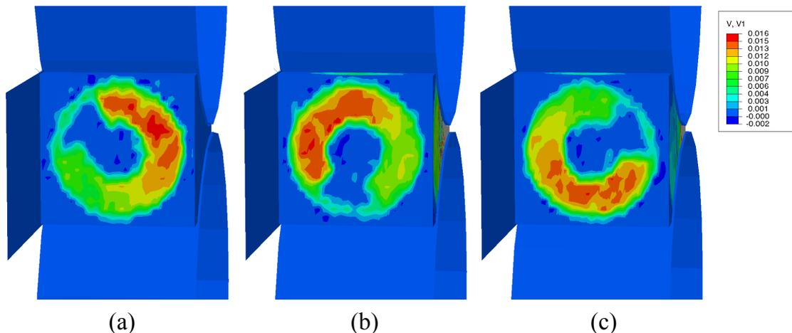
Figure 4.11: 3D plots of the axial velocity component  $\bar{v}_z$  in the FE model (right seal removed for better visualisation) for 3 screw positions, with a counter-clockwise rotation. The absolute time corresponding to each snapshot is: a)  $t^* = 0$ , b)  $t^* = T_S/3$  and c)  $t^* = 2T_S/3$ .
