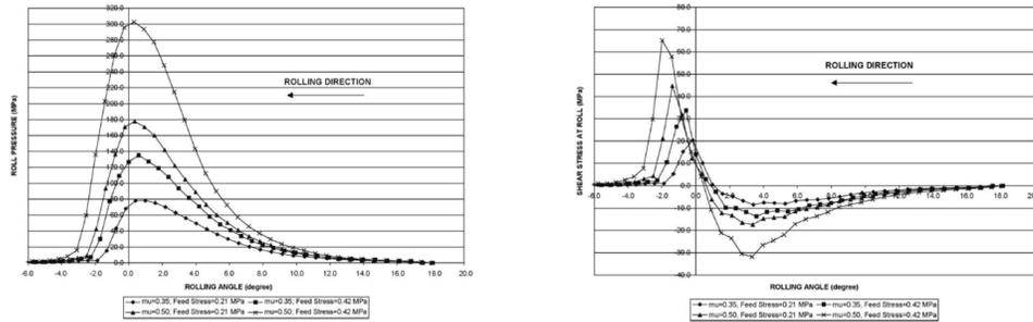
(a) Effect of friction on feed pressure on roll pressure (b) Effect of friction on feed pressure on roll shear stress
