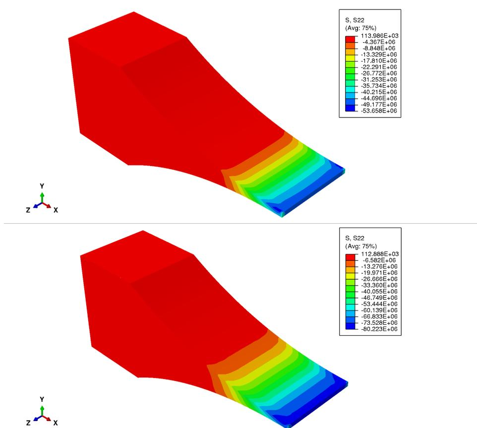
Figure 3.25: Resultant vertical stress,  $\sigma_{22}$  with a rimmed-roll for a)6 kN/cm and b)8 kN/cm roll separation force
