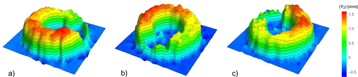
Figure 4.5: 3D plots of time-averaged CG axial velocity component computed for 3 screw positions. The absolute time corresponding to each snapshot is: a)  $t^* = 0$ , b)  $t^* = T_S/3$  and c)  $t^* = 2T_S/3$ .
