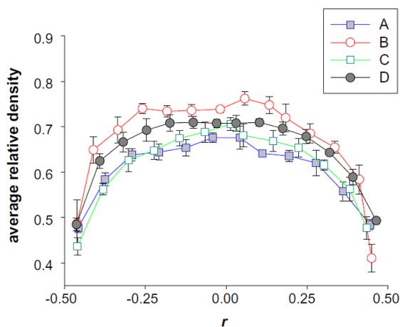
Figure 1.7: Density variation along the ribbon width obtained using micro-indentation with different roll gap (1mm (A,C,D) and 0.9 (B)) and roll speed (6 rpm (A,B) and 3 rpm (C,D)) [40]
