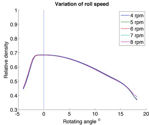
Figure 3.19: Effect of roll speed (using inlet feed pressure) on the relative density
