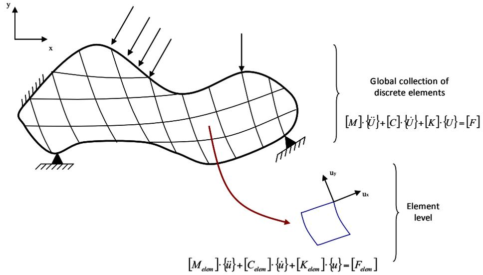
Figure 1.22: FEM global and element level relation
