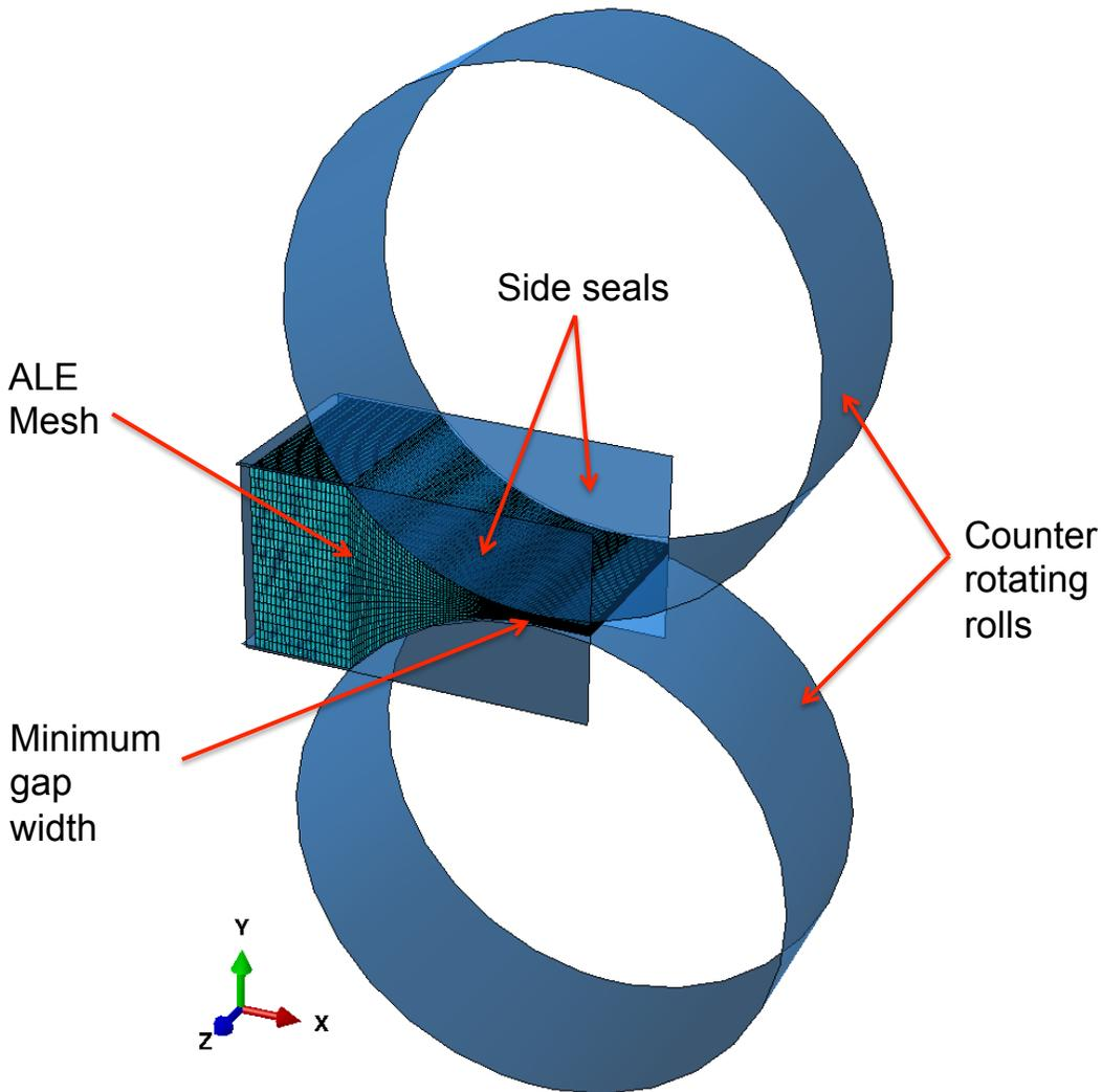
Figure 2.3: Schematic description of a typical FE model of roll compaction
