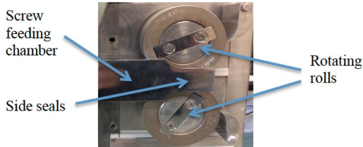
Figure 1.2: Side view of roll compactor Komarek B050H
