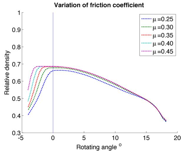
Figure 3.16: Effect of friction coefficient on the powder's relative density
