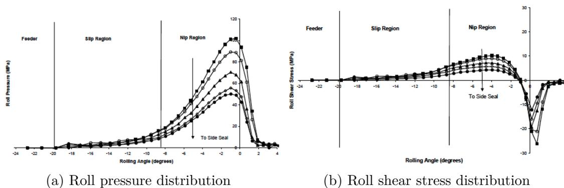
Figure 1.19: Three-dimensional FEM simulation results by Cunningham et al. [3]
