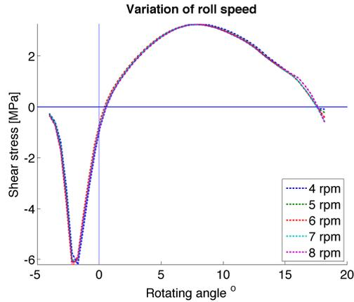
Figure 3.18: Effect of roll speed (using inlet feed pressure) on the shear stress
