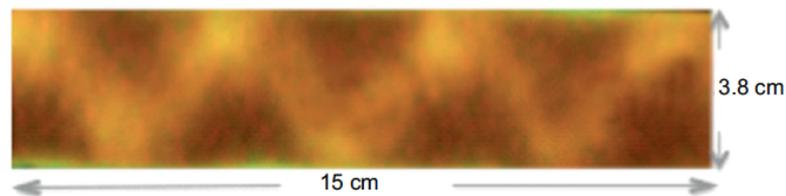
Figure 1.10: Results of light transmission through the depth of MCC ribbon [9]
