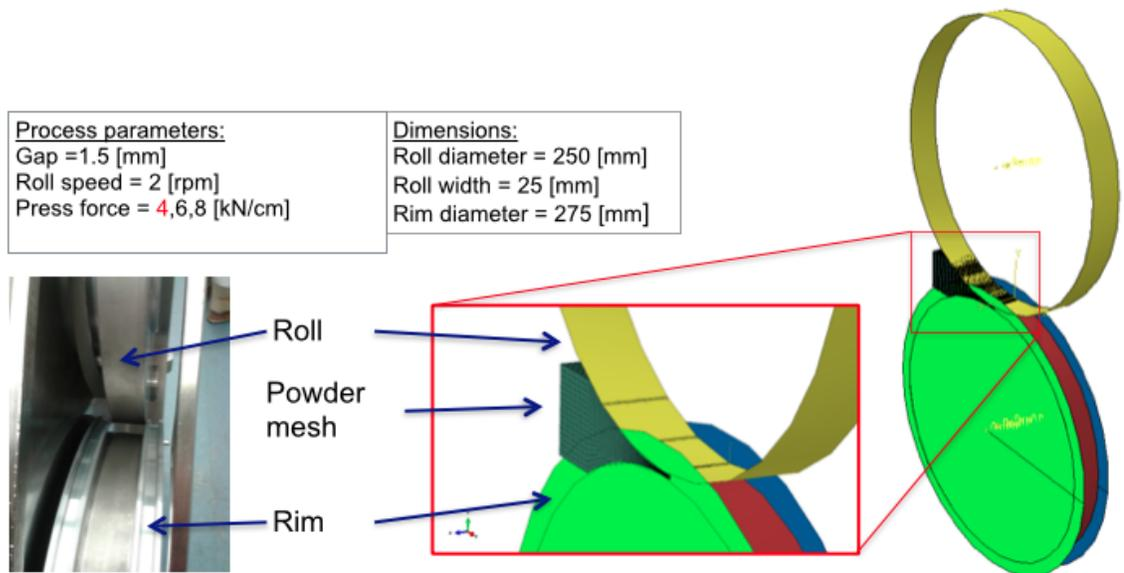
Figure 3.24: Detailed description of FE model using rimmed-roll sealing system
