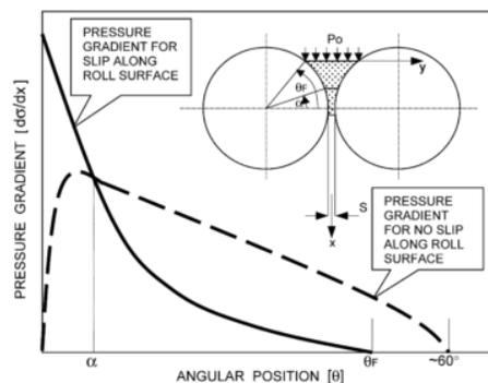
Figure 1.13: Vertical pressure gradient vs. angular position in roll bite [6]
