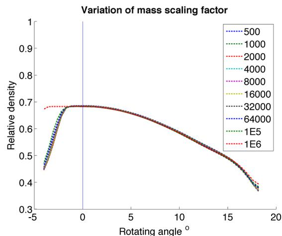
Figure 3.7: Effect of mass scaling on powder relative density along rolling direction
