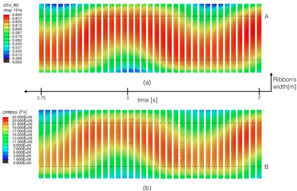
Figure 4.15: Multiple sliced snapshots of the a) relative density and b) contact pressure values obtained by the combined DEM-FEM simulations at the minimum gap region between  $t = 2.00s$  and  $t = 3.75s$ . The two highlighted positions A and B are the positions where the values of figure 4.14 are evaluated.
