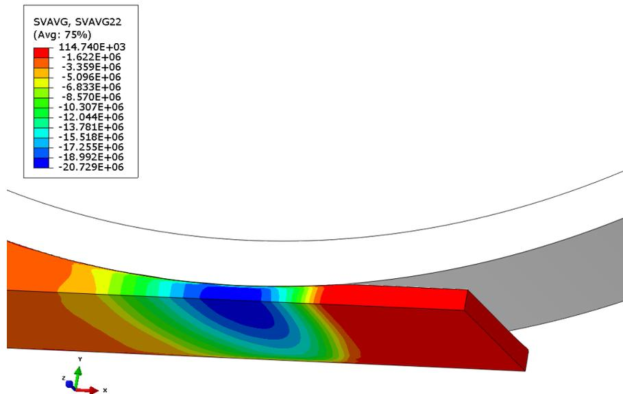
Figure 5.6: Vertical stresses,  $\sigma_{yy}$  on the fourth-folded symmetry model
