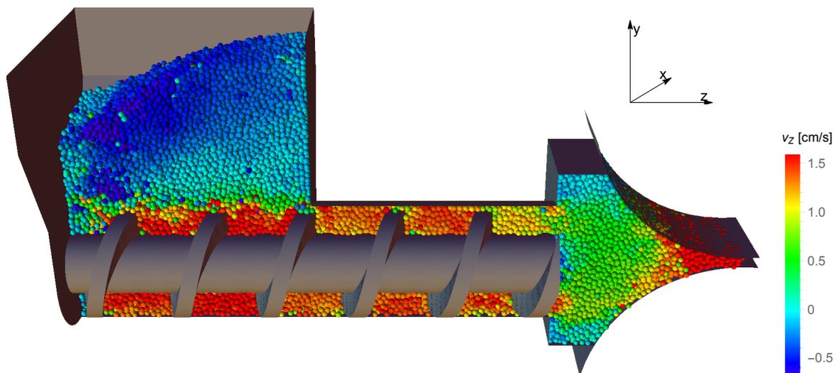
Figure 4.2: Vertical section of one snapshot of the system at steady-state, the particles are coloured according to their axial velocity  $v_z$ .
