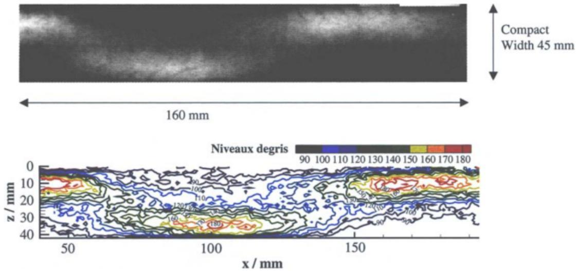
Figure 1.9: Light transmission through a sodium chloride ribbon (top) and iso-levels of the light transmission (bottom) [47]
