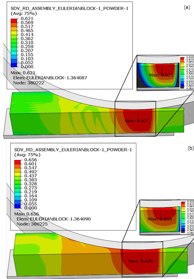
Figure 5.9: Resultant relative density for a given inlet velocity of a) 0.01 and b) 0.015 m/s.
