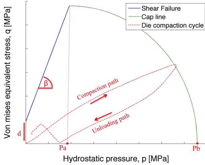
Figure 2.6: The Drucker-Prager Cap yield surface model in q-p plane.
