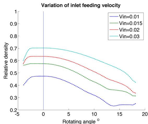
Figure 3.13: Effect of inlet feed velocity on the powder’s relative density
