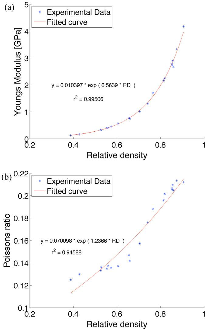
Figure 2.7: Elastic properties a) Young's Modulus,  $E$  and b) Poisson's ratio,  $\nu$
