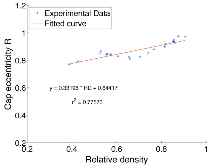
Figure 2.10: Cap eccentricity parameter R as function of relative density.
