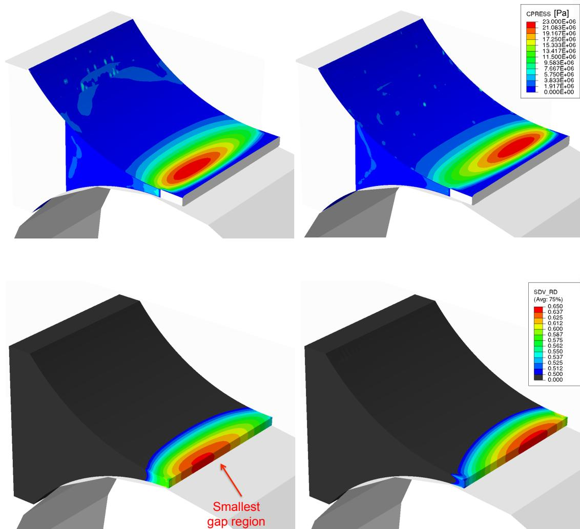
Figure 4.13: 3D FEM plots for 2 time steps:  $t^* = 2.35s$  (left column) and  $t^* = 2.9s$  (right column). The depicted values are: powder contact pressure (top row) and relative density (bottom row) at the outlet of the compaction region.
