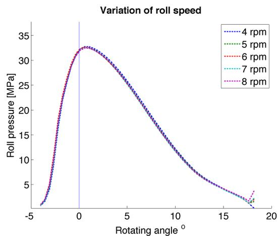
Figure 3.17: Effect of roll speed (using inlet feed pressure) on the roll pressure
