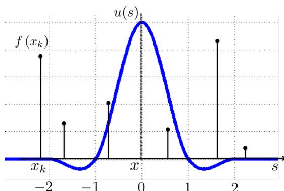
Figure 4.6: Interpolation kernel proposed by R.Keys [91]
