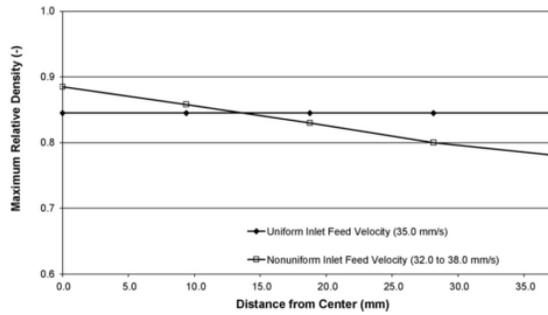
Figure 1.20: Density distribution along the ribbon width for two cases of inlet feeding velocity[3]
