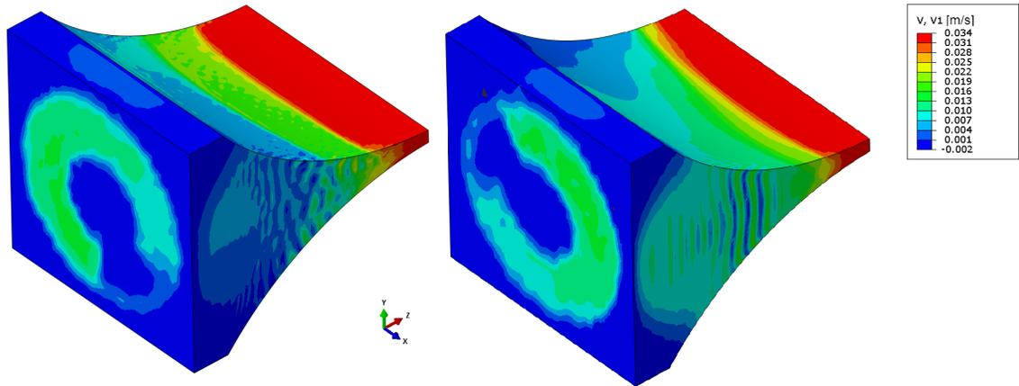
Figure 4.12: 3D FEM plots of powder axial velocity for 2 time steps:  $t^* = 2.35s$  (left column) and  $t^* = 2.9s$  (right column)
