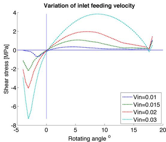
Figure 3.12: Effect of inlet feed velocity on the shear stress
