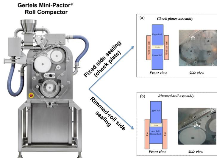
Figure 2.1: Gerteis Mini-factor's two possible side seal assemblies a)cheek plates b)rimmed-roll.
