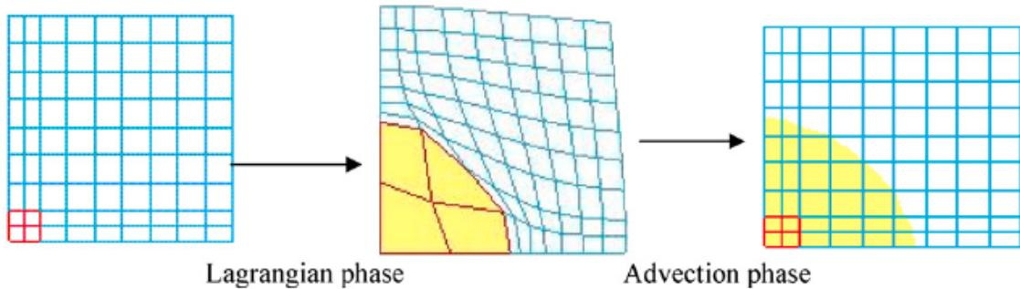
Figure 1.27: Lagrangian and Advection phases in ALE formulation [60]
