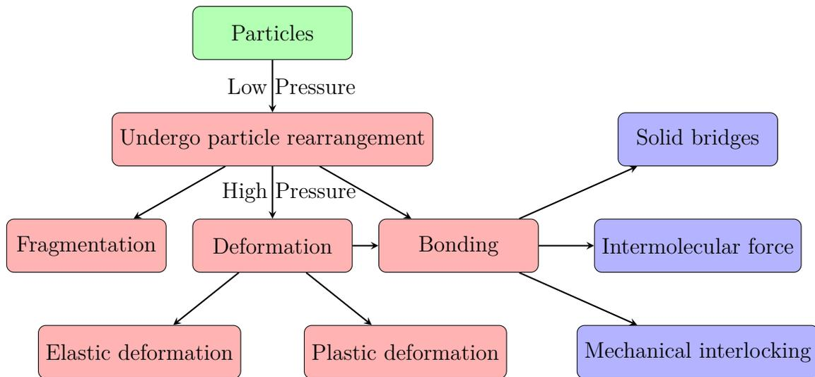
Figure 1.4: Flowchart of powder compaction
