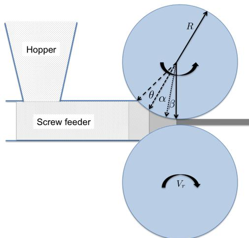
Figure 1.6: Schematic representation of roll compaction represented by three angles under the rolls.
