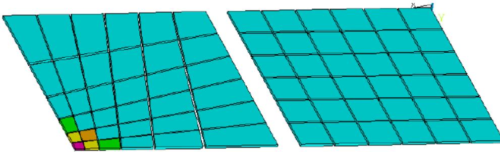
Figure 1.25: Different element sizes influence on mass scaling
