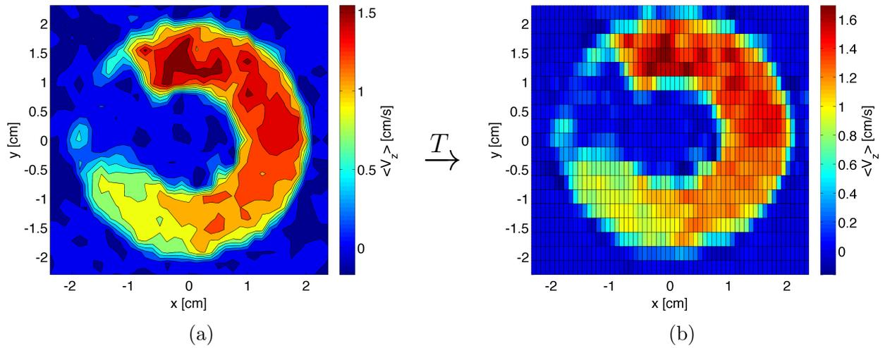
Figure 4.8: Plot of velocity field and the transition from CG result to FEM inlet boundary condition for  $t^* = 0$ . Axial velocity component  $\bar{v}_z$  values for a) DEM coarse graining result and b) Corresponding FE inlet nodes.
