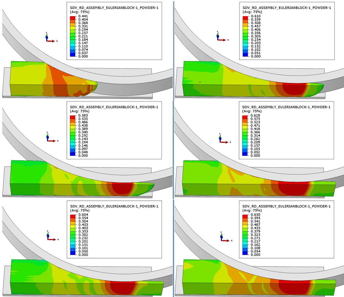
Figure 5.11: Comparison of powder relative density in CEL FE model
