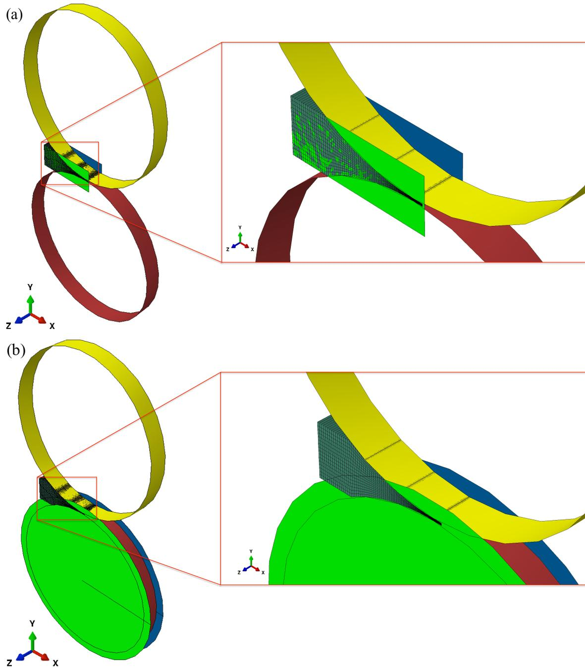
Figure 3.23: FE models of roll compactor with a)cheek plates and b)rimmed-roll
