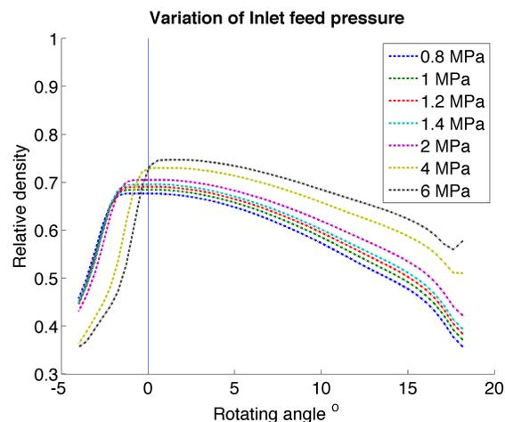
Figure 3.10: Effect of inlet feed pressure on the powder's relative density
