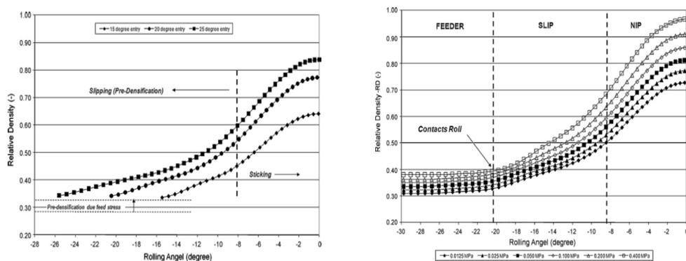
(a) Effect of powder entry angle on relative density in rolling direction (b) Effect of inlet feeding pressure on relative density in rolling direction
