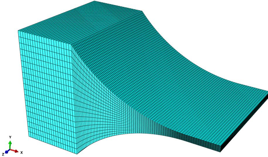
Figure 2.5: Discretized mesh of the powder region in the FE model
