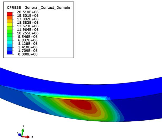
Figure 5.7: Resultant roll contact pressure in CEL FEM model
