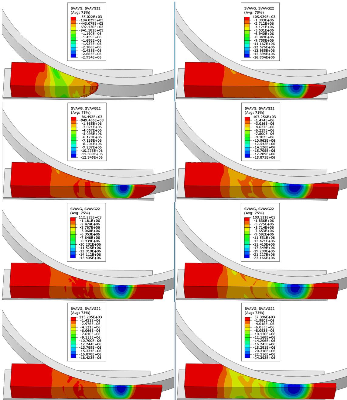
Figure 5.10: Comparison of vertical stress,  $\sigma_{22}$  in CEL FE model
