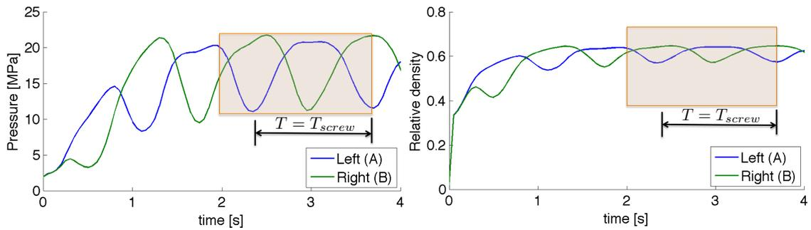
Figure 4.14: Plots of the a) roll contact pressure and b) relative density at two positions 5mm from both edges with respect of time. The highlighted region is the time domain used for plotting figure 4.15
