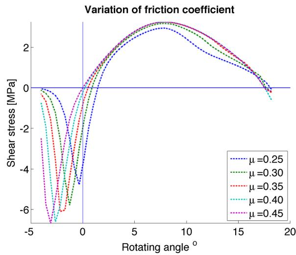
Figure 3.15: Effect of friction coefficient on the shear stress
