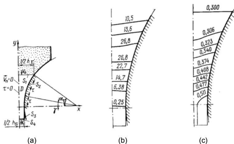
Figure 1.14: BVP solved by G. Gun et al, starting from a) describing the problem and obtaining the resultant field of isolines of b) deformation rate intensity and c) relative density [57].
