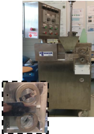
Figure 2.2: The Komarek B050H laboratory roll compactor
