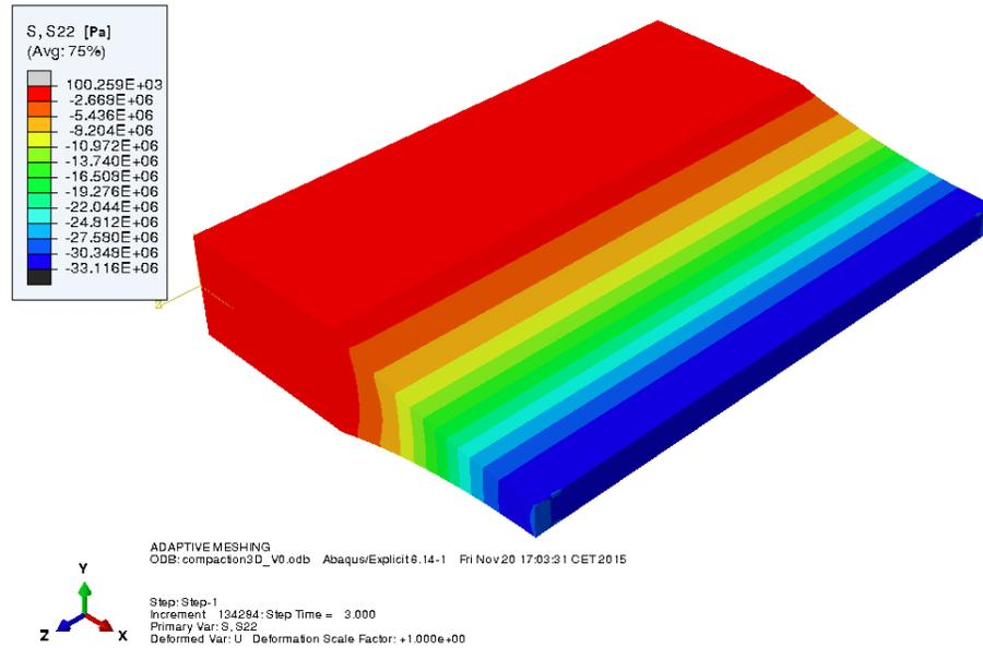
Figure 3.4: Reference FEM model results of vertical stress,  $\sigma_{22}$
