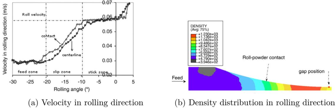
Figure 1.16: Two-dimensional FEM simulation results by Michrafy et al. [4]
