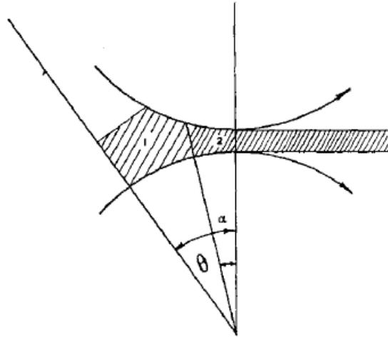
Figure 1.5: Schematic representation of roll compaction. Zone 1: incoherent powder; zone 2: coherent powder [33].
