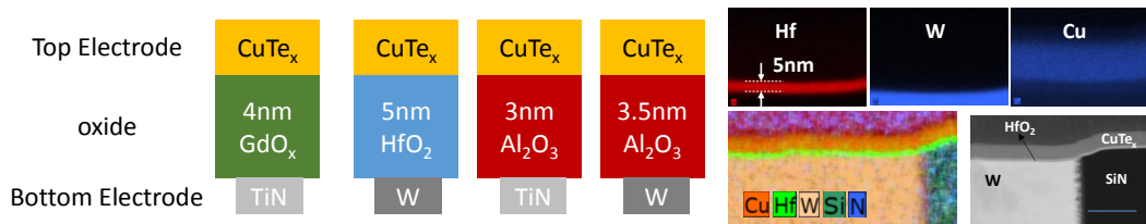
Figure 5.2: Schematic of the RRAM technologies studied in this work with TEM cross sections of \text{W/HfO}_2/\text{CuTe}_x based CBRAM, and EDX (Hf, W, Cu) images.
