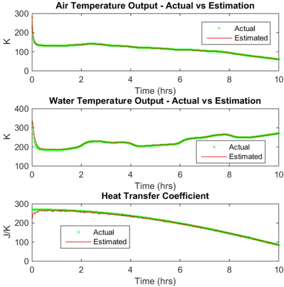
Figure 2.2: State and parameter estimates:  $U_A$  estimation (Example 1)
