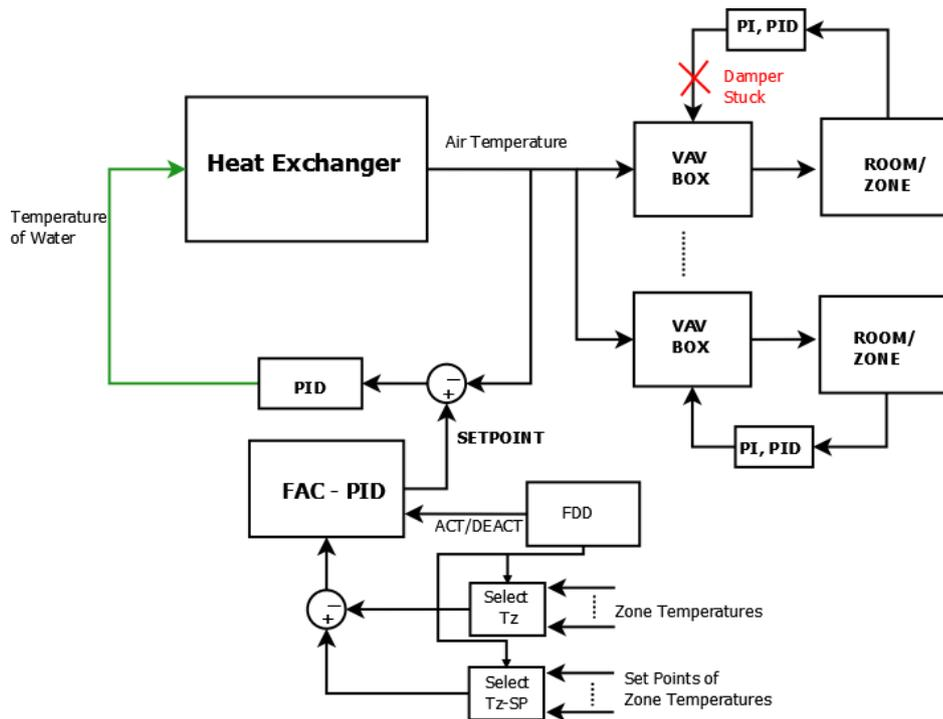
Figure 1.6: Schematic of fault adaptation strategy for the damper stuck fault
