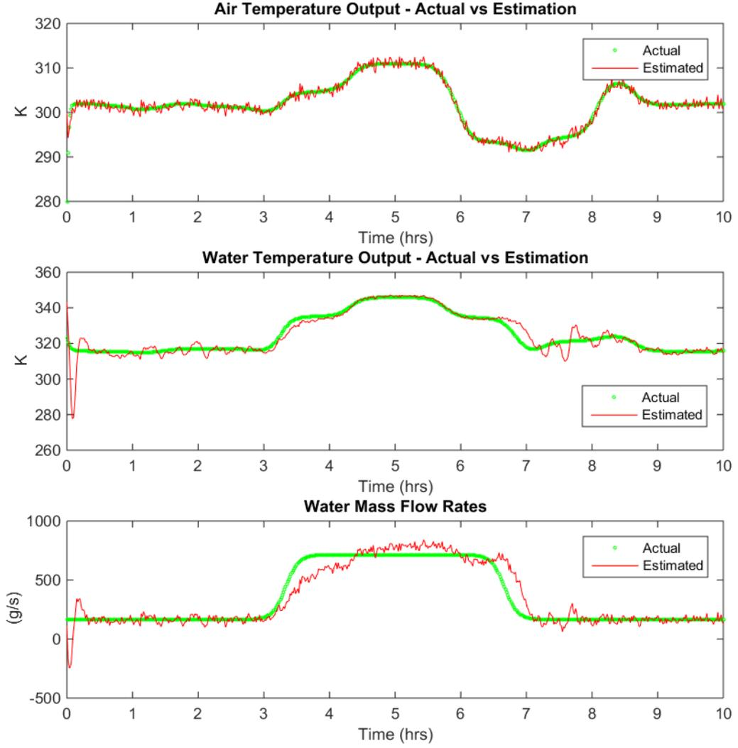
Figure 2.4: State and parameter estimates:  $q_w$  estimation (Example 3)
