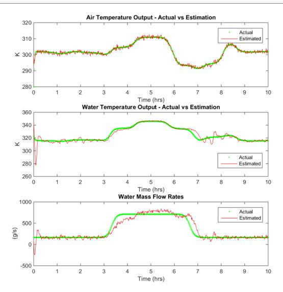
Figure 2.4: State and parameter estimates:  $q_w$  estimation (Example 3)
