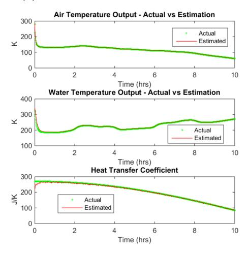
Figure 2.2: State and parameter estimates:  $U_A$  estimation (Example 1)
