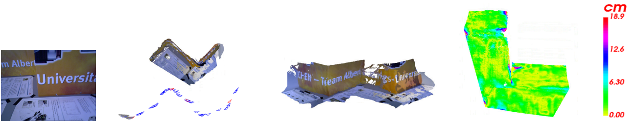
(b) Sequence “ fr3:structure_texture_near ”. Right:Euclidean distances with respect to ground truth of image sample on left (top view).
