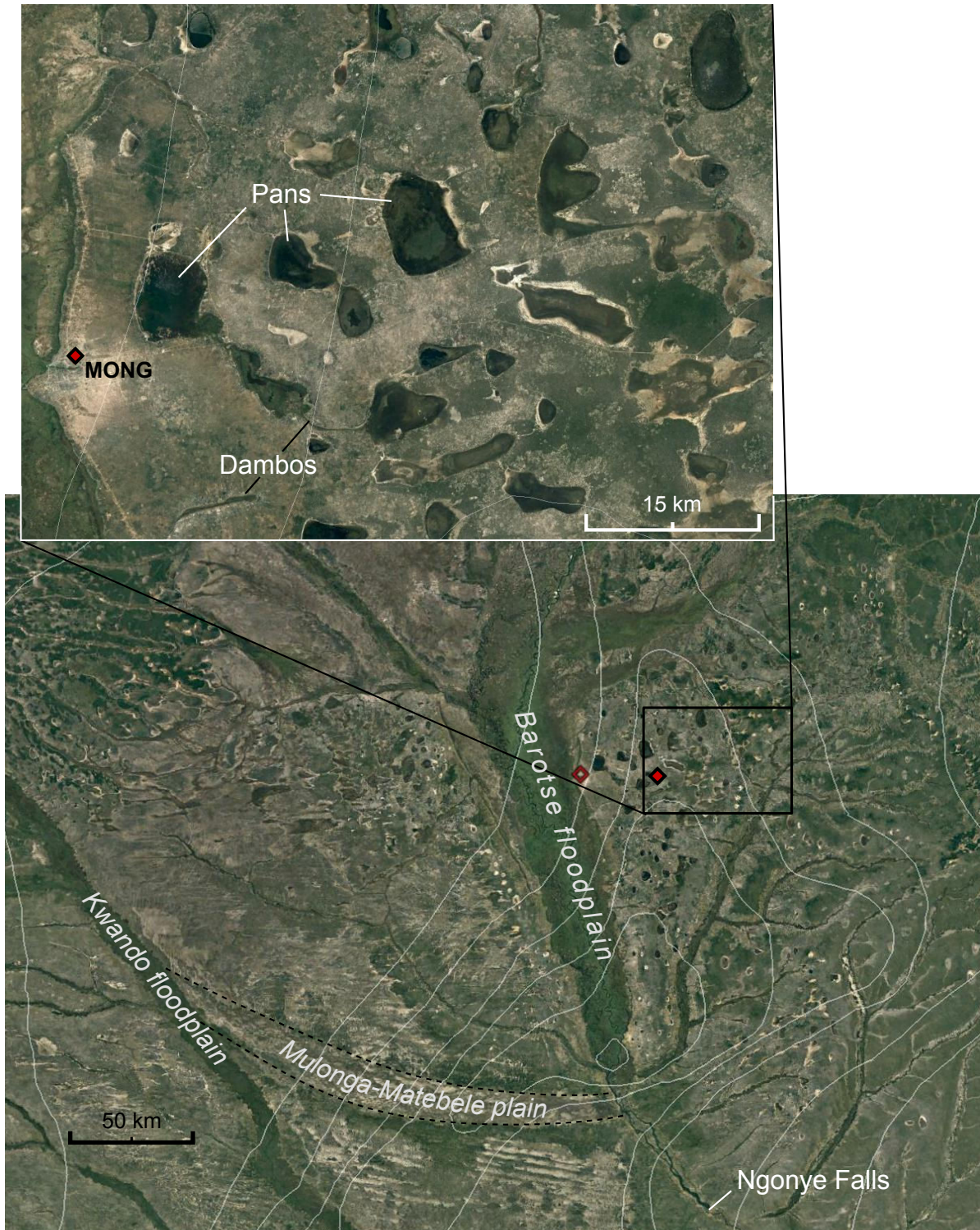
FIGURE 4.6 – Satellite views of the region of Mongu (Zambia). Bottom image shows the numerous geomorphological features of important groundwater storage with the extensive Barotse floodplain hosting the Upper Zambezi surrounded by seasonal to perennial pans and fed by several dambos. Top image shows a detailed view of pans and dambos (Source : Landsat/Copernicus by Google Earth).
