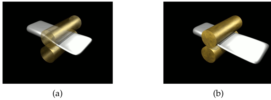
FIGURE 4.1 – Passage of strip through work rolls
