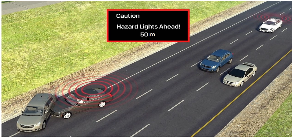
Figure 2.2: Accident detection by using V2V communication.
