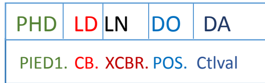
Figure 2.11 : The concept of physical device with path to data attributes of logical nodes
