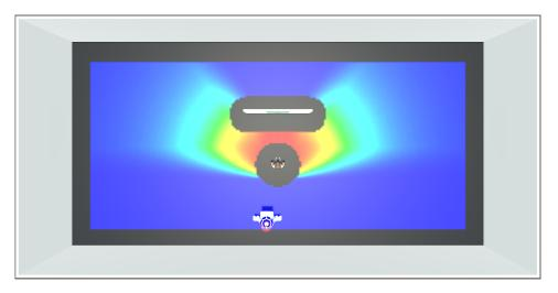
Figure 3.10: Illustration of an attention field in a scenario featuring a person watching a painting (the warmer the color the highest the value). The attention field is not defined in unfeasible regions for the robot (i.e. regions where a collision would occur).
