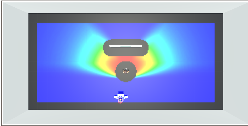
Figure 3.10: Illustration of an attention field in a scenario featuring a person watching a painting (the warmer the color the highest the value). The attention field is not defined in unfeasible regions for the robot (i.e. regions where a collision would occur).
