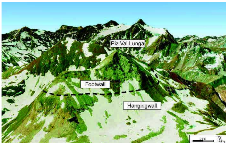
Fig. 4.1 - Panoramic view of Piz Val Lunga area. The dashed line marks the extensional detachment fault separating the extensional allochthon (hangingwall) and the Albula granite (footwall).
