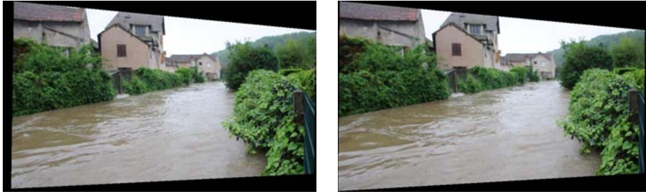
Figure 3.15: Rectified image pair using epipolar geometry, the camera motion causes points to only move on their corresponding epipolar lines which are parallel to x axis in the rectified images.
