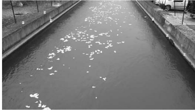
Figure 4.2: GRPs deployed on Claix canal.
