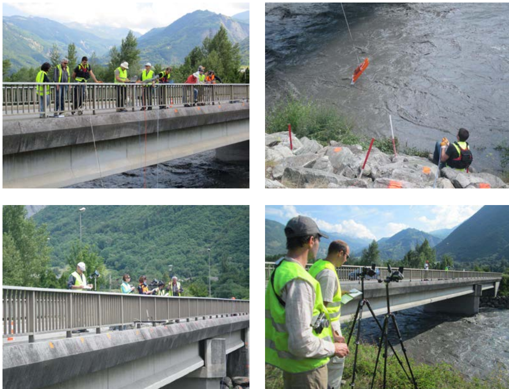
Figure 1.2: Velocity estimation techniques: Intrusive (top), radar-based (bottom left) and image-based (bottom right).
