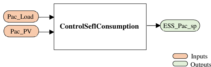
Figure 7-6. The basic ‘ControlSelfConsumption’ component structure
