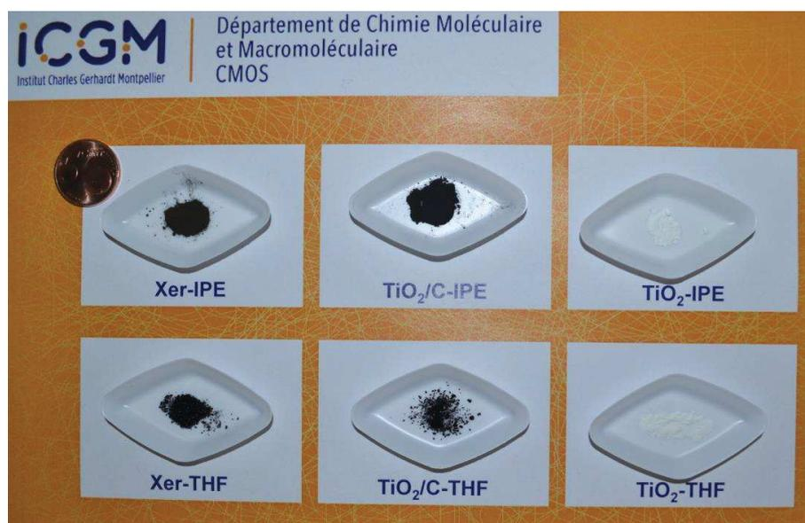
Figure 2.7 Picture of the IPE and THF derived TiO<sub>2</sub> xerogels and final products after heat treatment.
