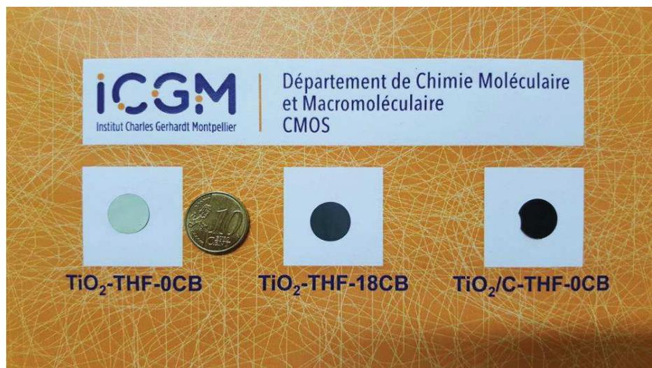
Figure 2.9 Visual aspect of TiO<sub>2</sub>-THF electrodes with and without acetylene black.
