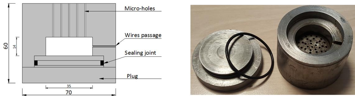
Figure 2.13: Drainage cap with micro-holes, plug and sealing joint (left) design (right) real concept
