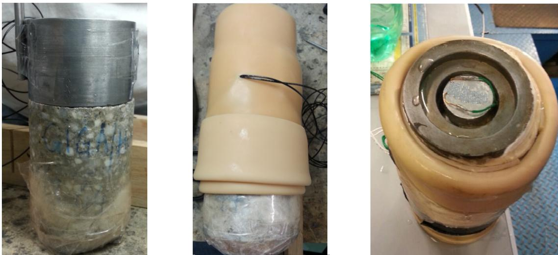
Figure 3.5: Experimental procedure: (left) sponge attached on concrete lower surface (middle) applying of protective membranes (right) saturation of the water collecting cap before the test
