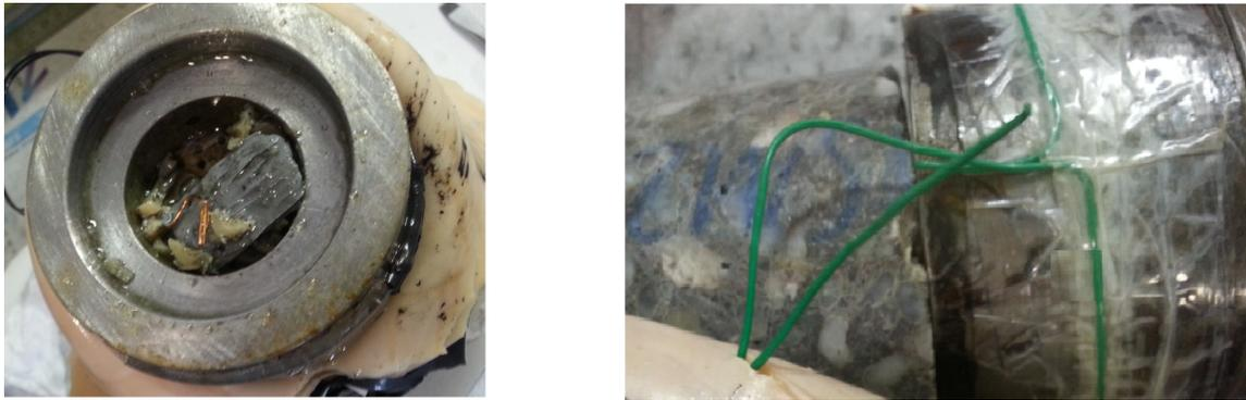
Figure 3.6: Device weak points: (left) membrane penetration (right) wires cut at cap/specimen interface
