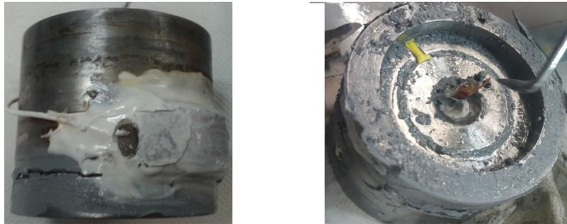
Figure 3.31: Lost of diaphragm pattern: (left) wires cut (right) gage detached
