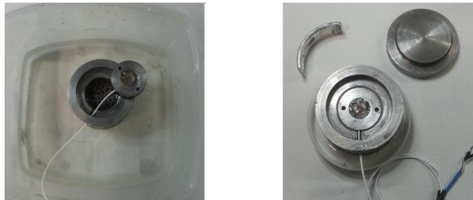
Figure 3.26: Test preparation: (left) cap saturation (right) sensor insertion
