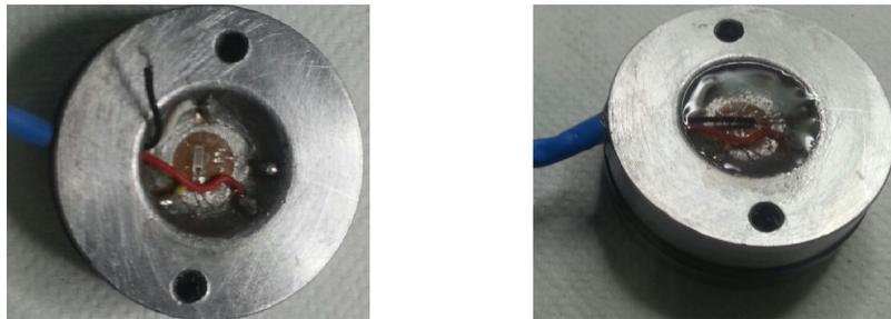
Figure 3.32: Single radial gage: (left) support and cosse gluing with wires welding (right) gage protection
