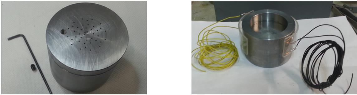
Figure 3.38: Water collecting cap with membrane effect: (left) real photo (right) gage application
