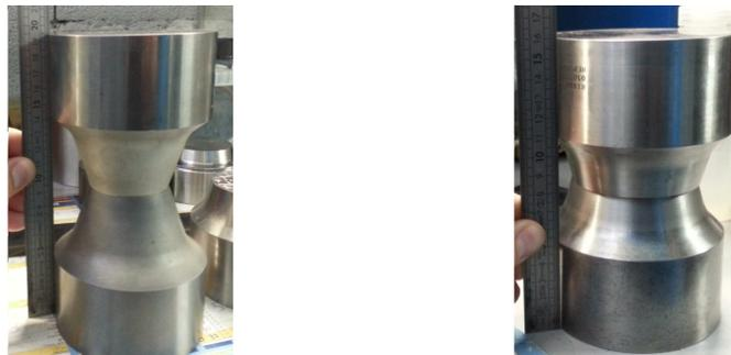
Figure 2.10: Principal caps dimensions and shapes adapted for both sample lengths and diameters: (a) 10.5 by 5 cm (b) 14 by 7 cm
