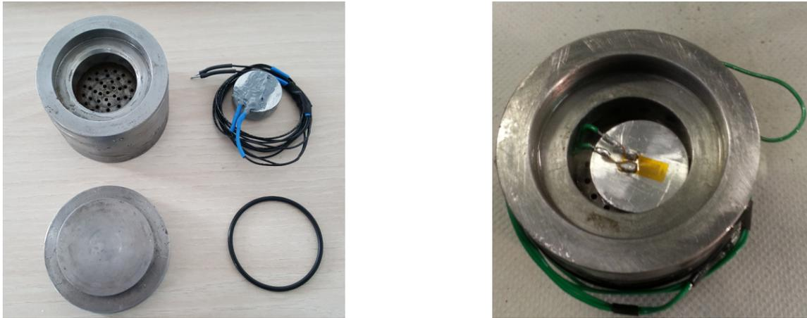
Figure 3.2: Picture of the aluminum sensor type hydrostatic: (left) water collect cap, plug, sealing joint and the hydrostatic sensor (right) sensor placed inside the water collecting cap
