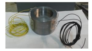
Figure 3.38: Water collecting cap with membrane effect: (left) real photo (right) gage application
