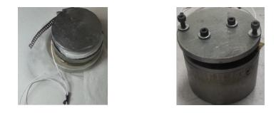
Figure 3.27: Test preparation: (left) application of the wires protective metal clamp shield (right) sensor lifting device
