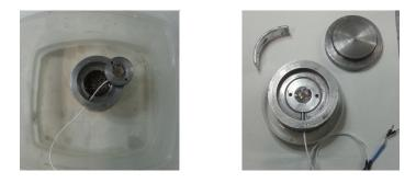
Figure 3.26: Test preparation: (left) cap saturation (right) sensor insertion
