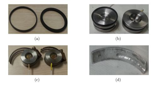
Figure 3.25: Sensor protection (a) joints made of two sub-items (b) joint insertion (c) application of the metal clamp (d) aluminum grooved shield
