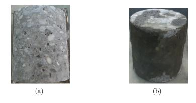
Figure 2.15: concrete surface porosity and *Sikatop* application: (a) before (b) after
