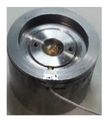
Figure 3.11: Steel sensor type membrane (a) sectional plan of the cap with the membrane sensor (b) picture of the cap with the membrane sensor
