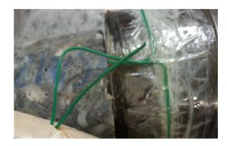
Figure 3.6: Device weak points: (left) membrane penetration (right) wires cut at cap/specimen interface
