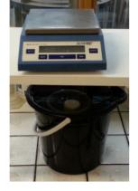
Weight of saturated sample immersed in water
