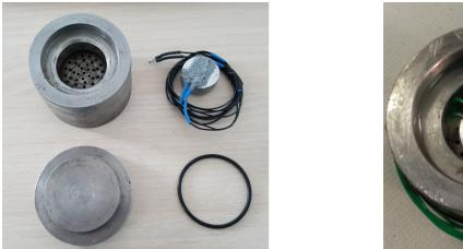
Figure 3.2: Picture of the aluminum sensor type hydrostatic: (left) water collect cap, plug, sealing joint and the hydrostatic sensor (right) sensor placed inside the water collecting cap
