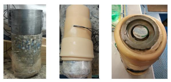
Figure 3.5: Experimental procedure: (left) sponge attached on concrete lower surface (middle) applying of protective membranes (right) saturation of the water collecting cap before the test
