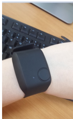
Fig. 5.1 A photo of the plugged E4 in the left hand of a driver. It is unobtrusive device allowing to perform the driving task.
