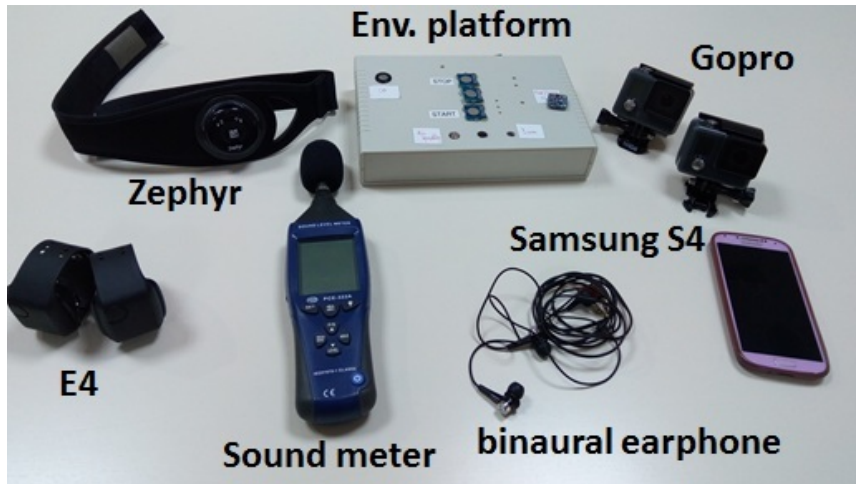
Fig. 5.4 An overview of the used sensors to capture the different signals
