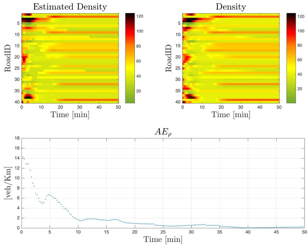
Figure 6.9: Density dynamic reconstruction: Ground truth (right) and estimated (left) time series in a RTN.
