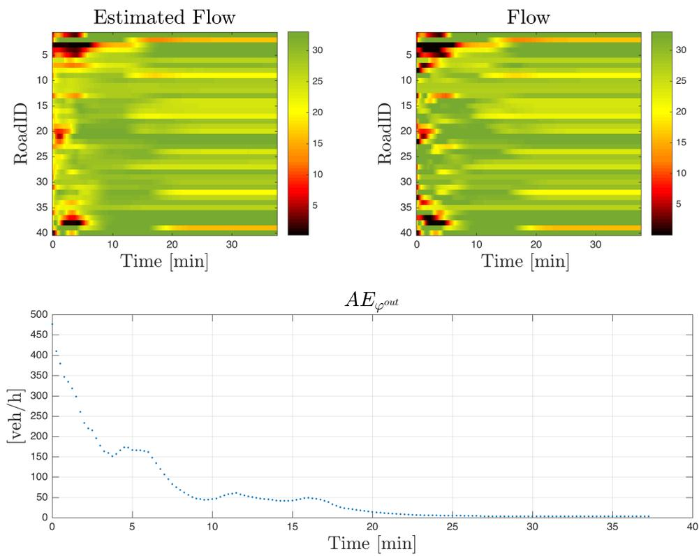
Figure 6.8: Flow dynamic reconstruction: Ground truth (right) and estimated (left) time series in a RTN.<sup>4</sup>
