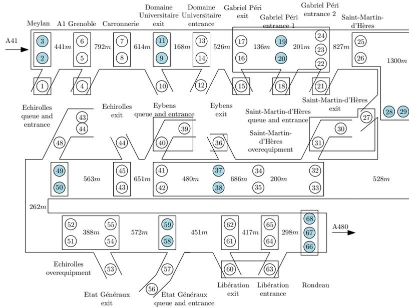
Figure 7.2: Detailed distribution of sensors within the Rociade Sud in the direction east-west. The positions of the 68 fixed sensor points are shown in the stylized map [LCK16].
