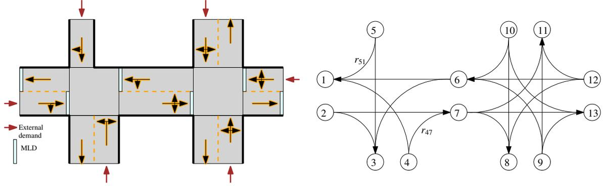
Figure 6.5: RTN and its graph model. Left hand side panel shows the physical infrastructure. Right hand side the graph  $\mathcal{H}$
