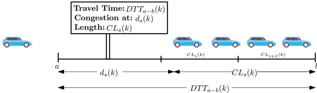
Figure 7.8: Speed panel indicators and displayed information. The panels display three main indicators  $DTT_{a-b}$ : travel time from the nearest origin to destination,  $d_s$ : and  $CL_s$  which represents the length of the congestion for a specific subset of sections
