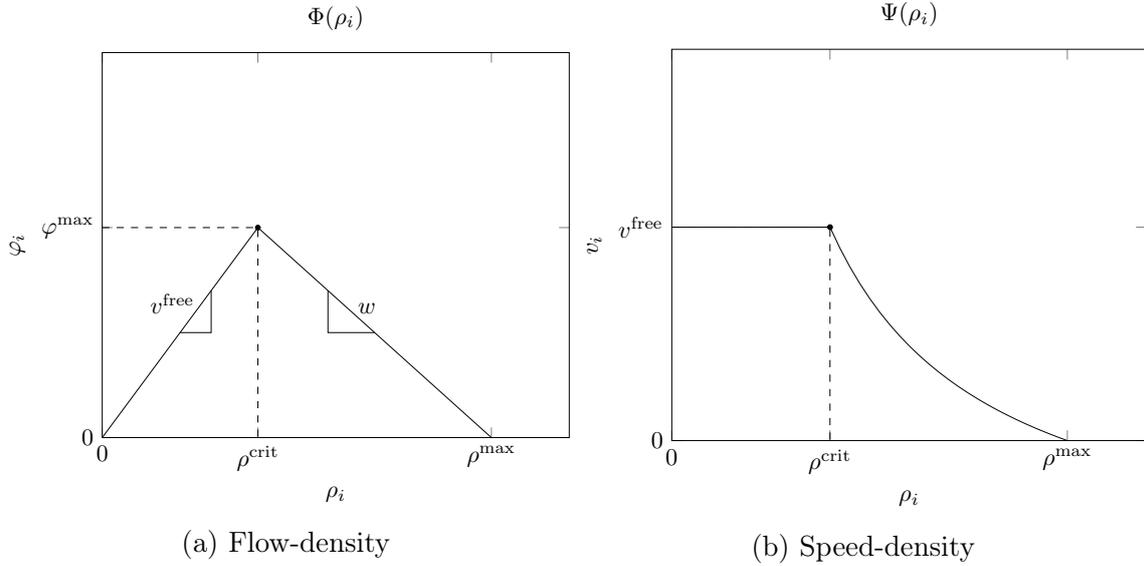
Figure 6.1: Density-flow and density-speed fundamental diagrams. The value of density  $\rho^{crit}$  is usually said *critical density*, and it represents the switching point between a free-flow regime and a congested one
