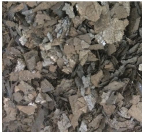
Figure 1.29. Cr 2 AlC platelet by one hour power ramp
