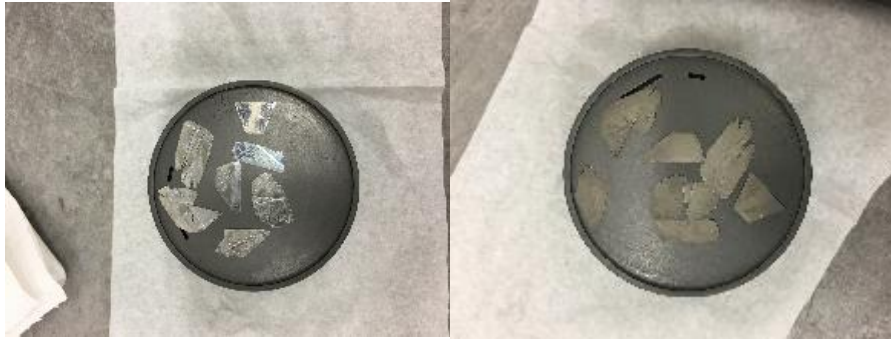
Figure 3.6. Crystal platelets (a) before and (b) after chlorination
