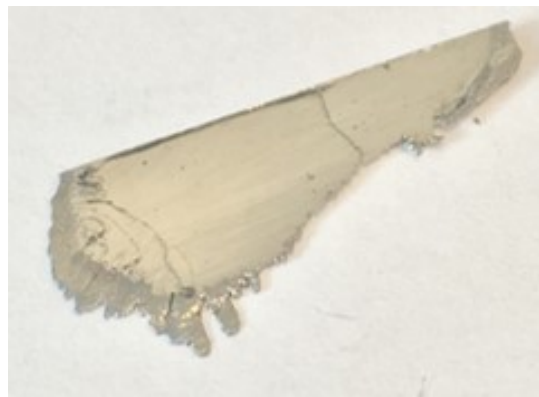
Figure 1.7. Cleaved surface of Cr 2 AlC single crystal
