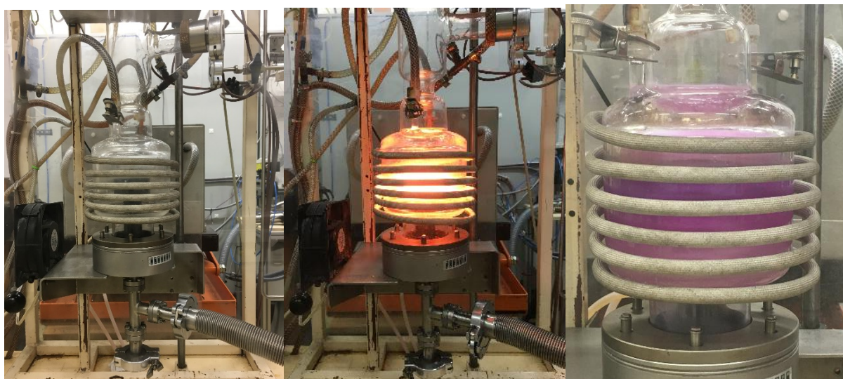
Figure 3.5. Reactor (a) before heating, (b) during heating and (c) after heating
