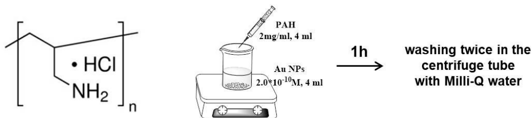
Scheme 3.3. Chemical structure of poly(allylamine hydrochloride) (PAH) (left) and schematic diagram of the procedure for Au NPs coating with PAH (right).
