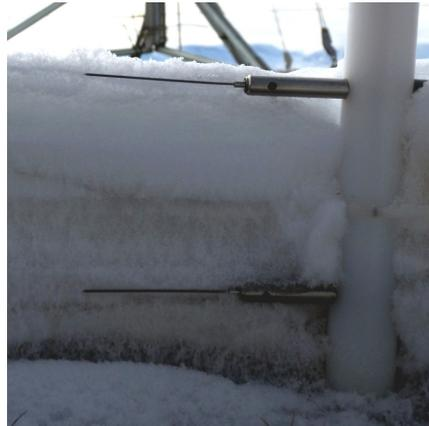
FIGURE 3.9 – Photograph of the snow stratigraphy taken on 14 May 2014. The NPs are 7 and 17 cm above the ground. The various depth hoar and indurated depth hoar layers between 0 and about 11 cm are clearly visible, as well as the wind slab between 11 and 16 cm.
