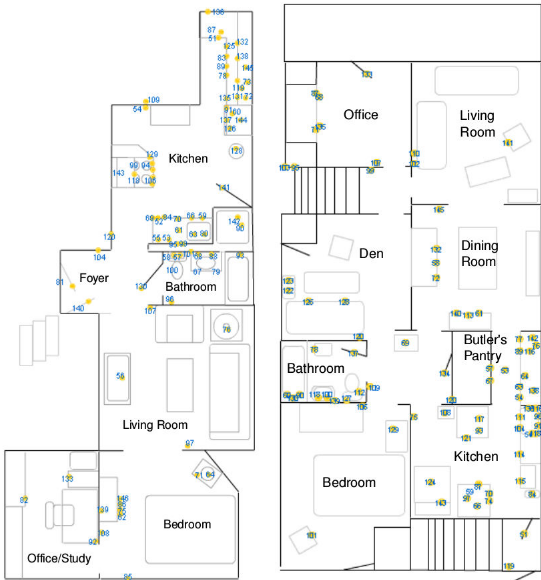
Figure 2.1.5: (a) The top view of the apartments and the sensor distribution for subject one. (b) Sensor distribution for subject two. Tapia et al. (2004) .
