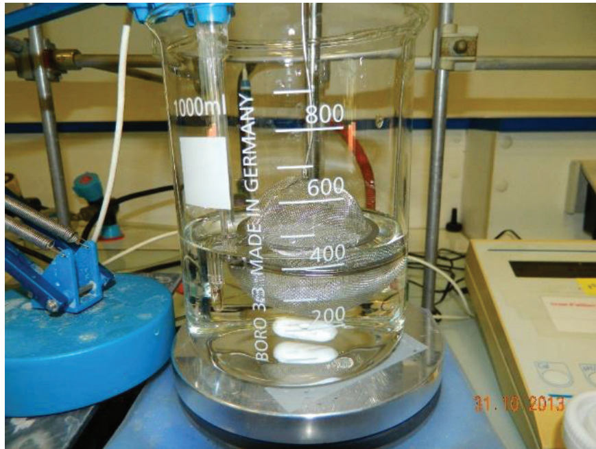
Figure 3.1. Experimental setup used for studying the diffusion coefficient in chitosan hydrogels (disk geometry)
