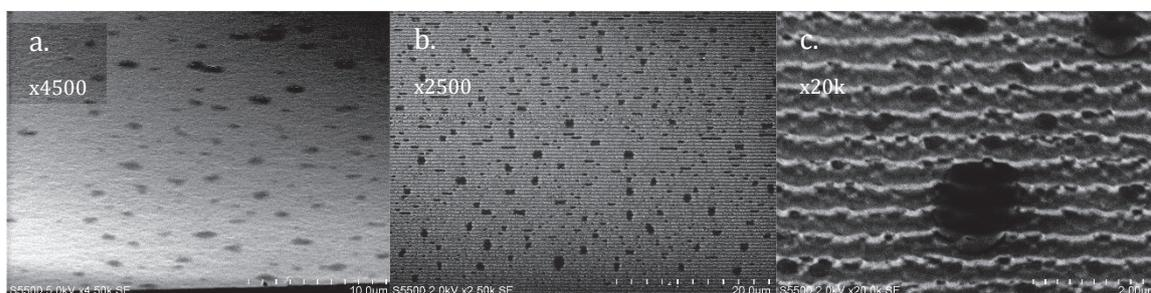
**Fig. IV.4** – MEB pictures of the bottom (a) and the sides (b-c) of the channel. Stationary phase does not form a continuous film but small beads (in dark in the pictures).
