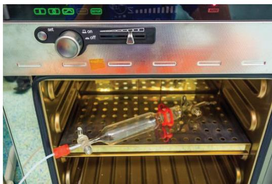
**Fig. A.5** – Picture of the glass container, placed into the oven for powder synthesis in “column like” conditions.
