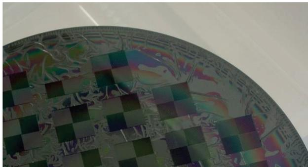
**Fig. V.19** – Picture of a wafer after the deposition of the first PEI layer.
