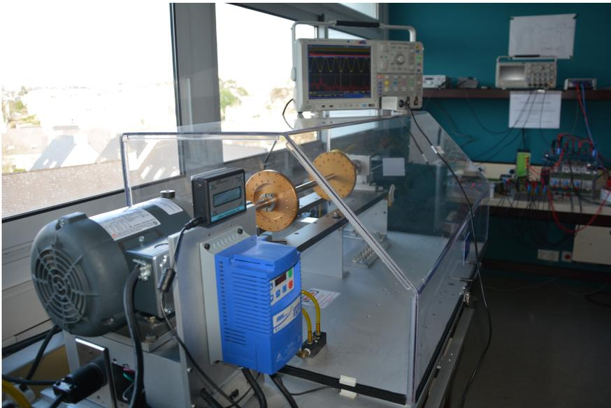
Figure 4.1: Machinery fault simulator.
