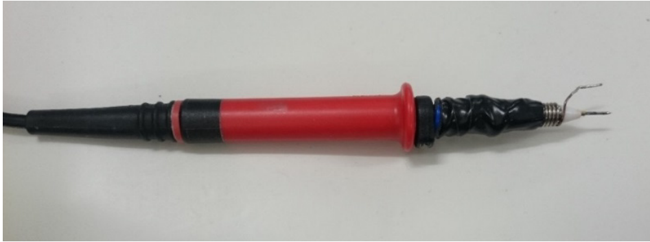
Fig. 2.22: The adjusted passive voltage probe
