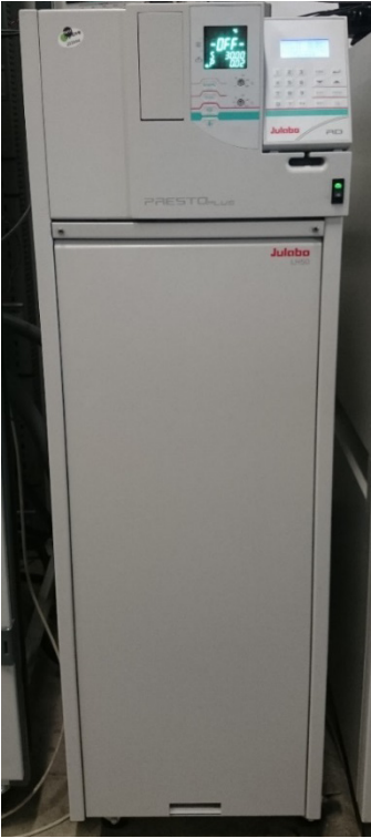
Fig. 5.9: LH50plus temperature regulation system
