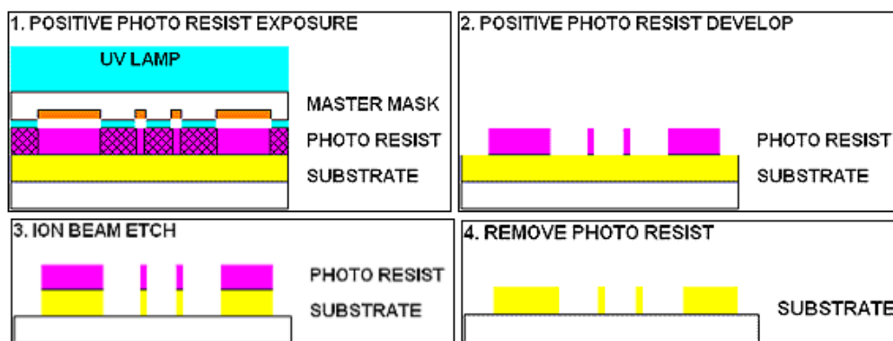
Figure 79 Schematic of IBE process. The figure is reproduced from the website of http://www.microfabnh.com/ion_beam_etch_technology.php
