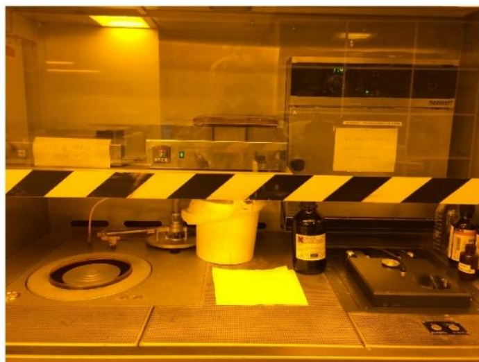
Figure 81 The spin-coating setup in C2N
