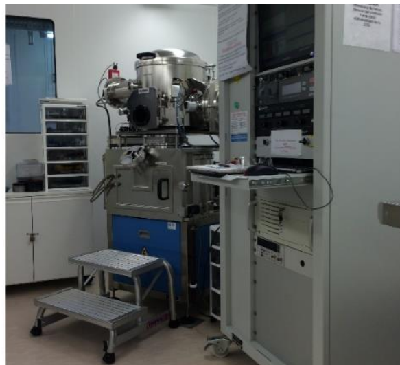
Figure 64 E-beam evaporation setup in C2N
