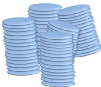
Figure 1.3. Schematic representation of the N_{\text{col}} phase of discotic liquid crystals.
