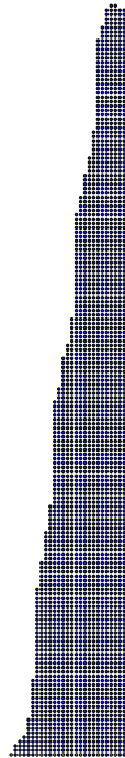
Figure 6.9: Example of bitheaps coming from FloPoCo's FixFIR operator, corresponding to a large FIR filter. The architecture of the filter is based on constant multiplications by the coefficients of the filter.
