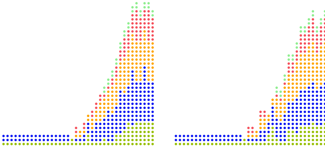
(c) The two bit heaps for 32-bit faithful results, using one DSP block for each multiplication.
