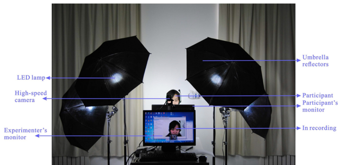
FIGURE 2.12: Acquisition setup for elicitation and recording of micro-expressions. Figure reprinted from [WJYWZ + 14].
