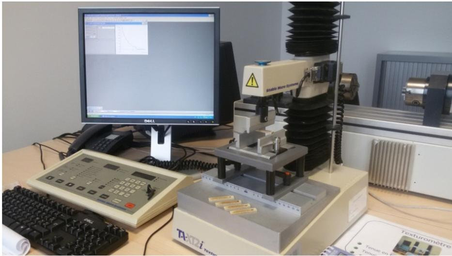
FIG. 3.15: machine de traction-compression.
