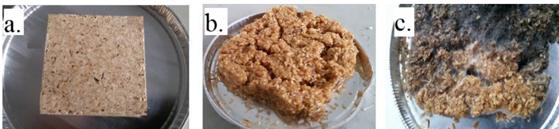
Fig. 8. The water effect on 100% hemp shive composites (a) before, (b) after immersion in water and (c) after 14 days of fermentation.
