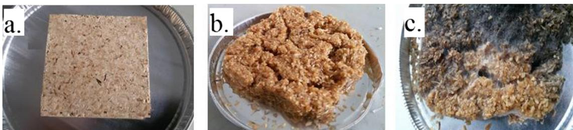
Fig. 8. The water effect on 100% hemp shive composites (a) before, (b) after immersion in water and (c) after 14 days of fermentation.
