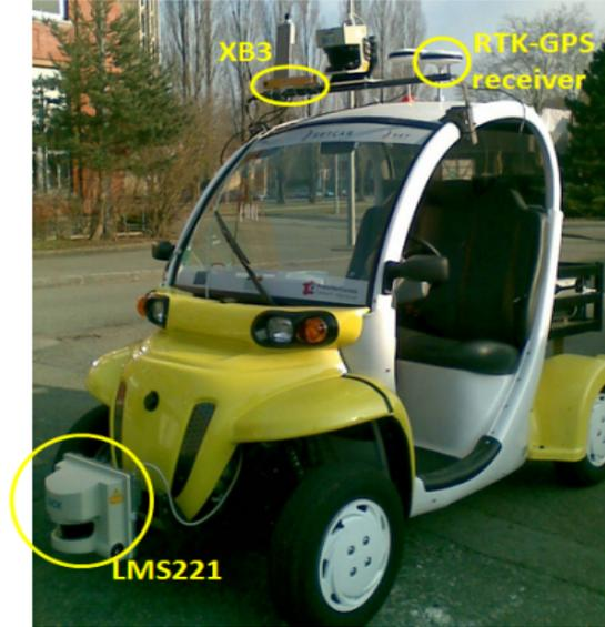
Figure 1-4: Experimental vehicle equipped with sensors (especially camera and RTK-GPS).
