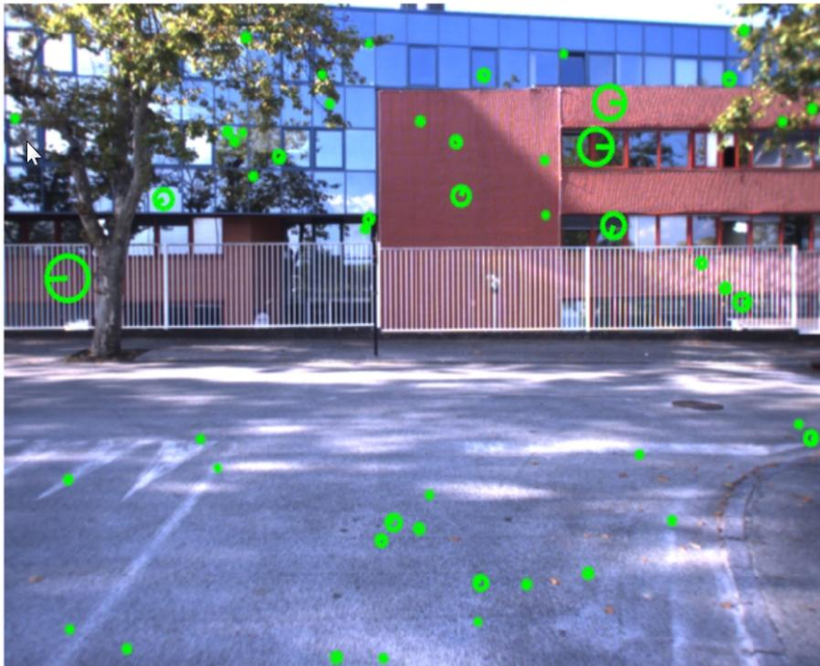
Figure 2-2: SIFT extracts interest points in an image for description. The circles are interest points selected by SIFT within the image. The number of possible features may vary depending on the number of interest points detected in the image.
